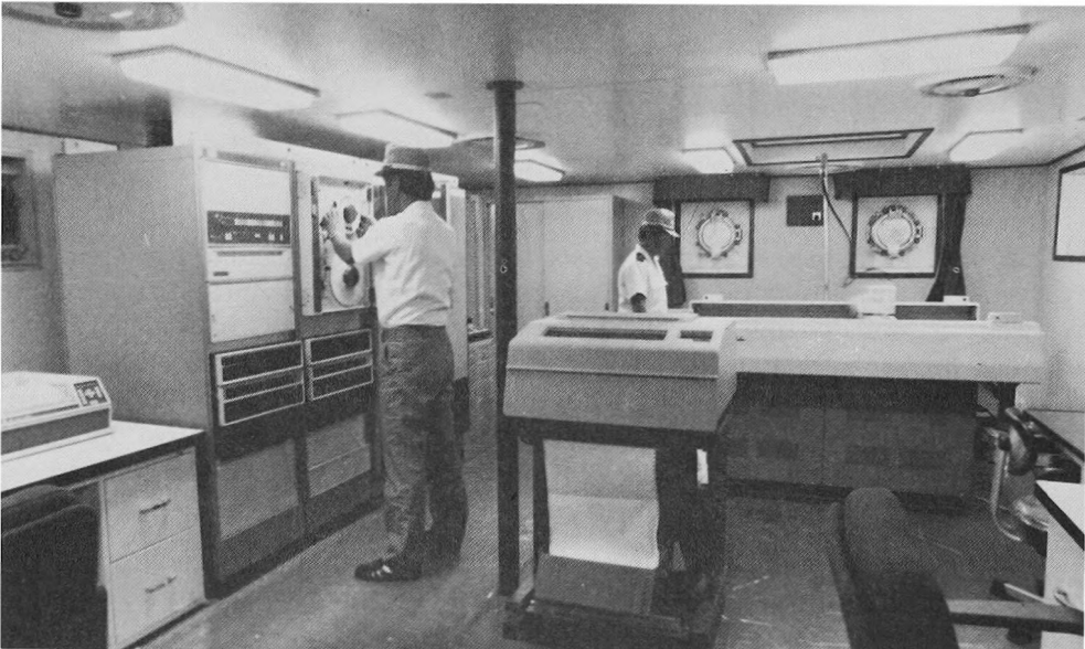
FIG. 5. — C.P.U., disc unit, MT unit and plotter in the computer room.
