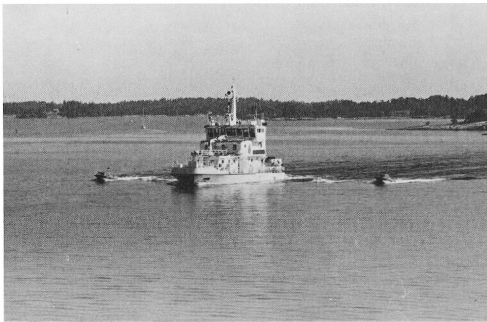
FIG. 2. — Surveying with booms and satellite boats.
