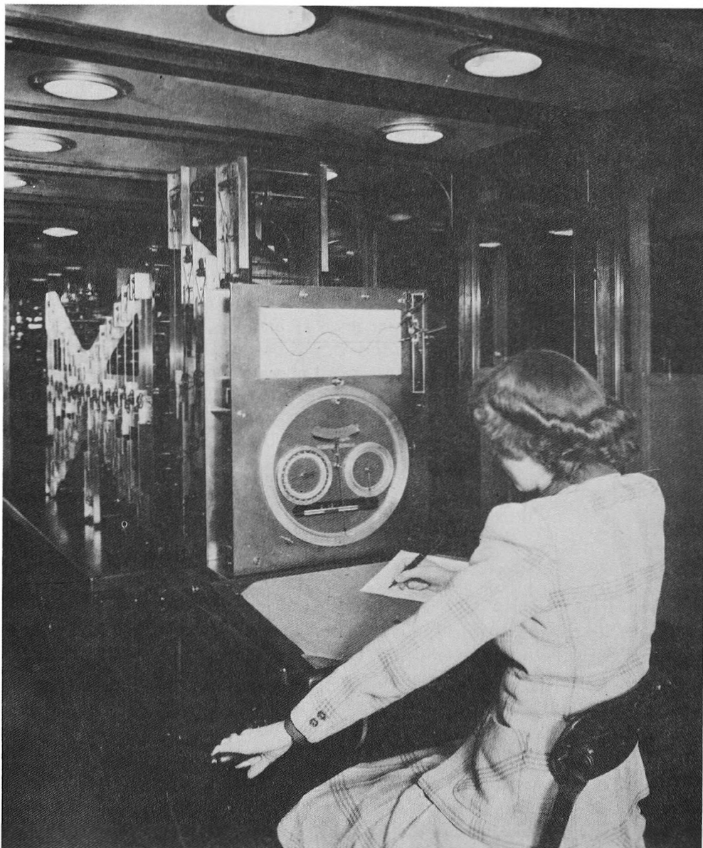
FIG. 1.— Second United States mechanical tide predicting machine used for predictions beginning in 1912. Using 37 constituents, its two banks of gears permitted obtaining both times and heights of high and low waters simultaneously and, in addition, it produced an inked curve of the prediction with marked times of high and low waters and hourly heights.
