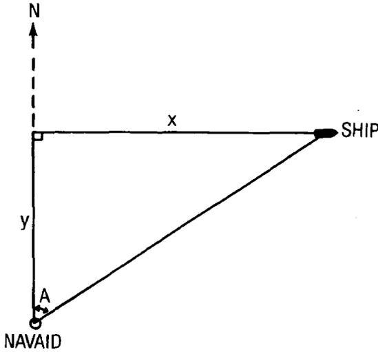
FIG. 2.— Plane triangle used for derivation of **B** matrix expression for the case of an azimuth navaid.
