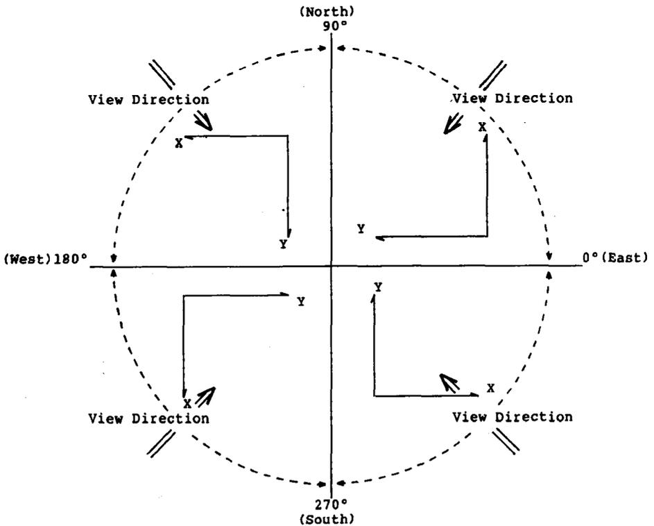
FIG. 6. — X-Y coordinates determined by view direction.
