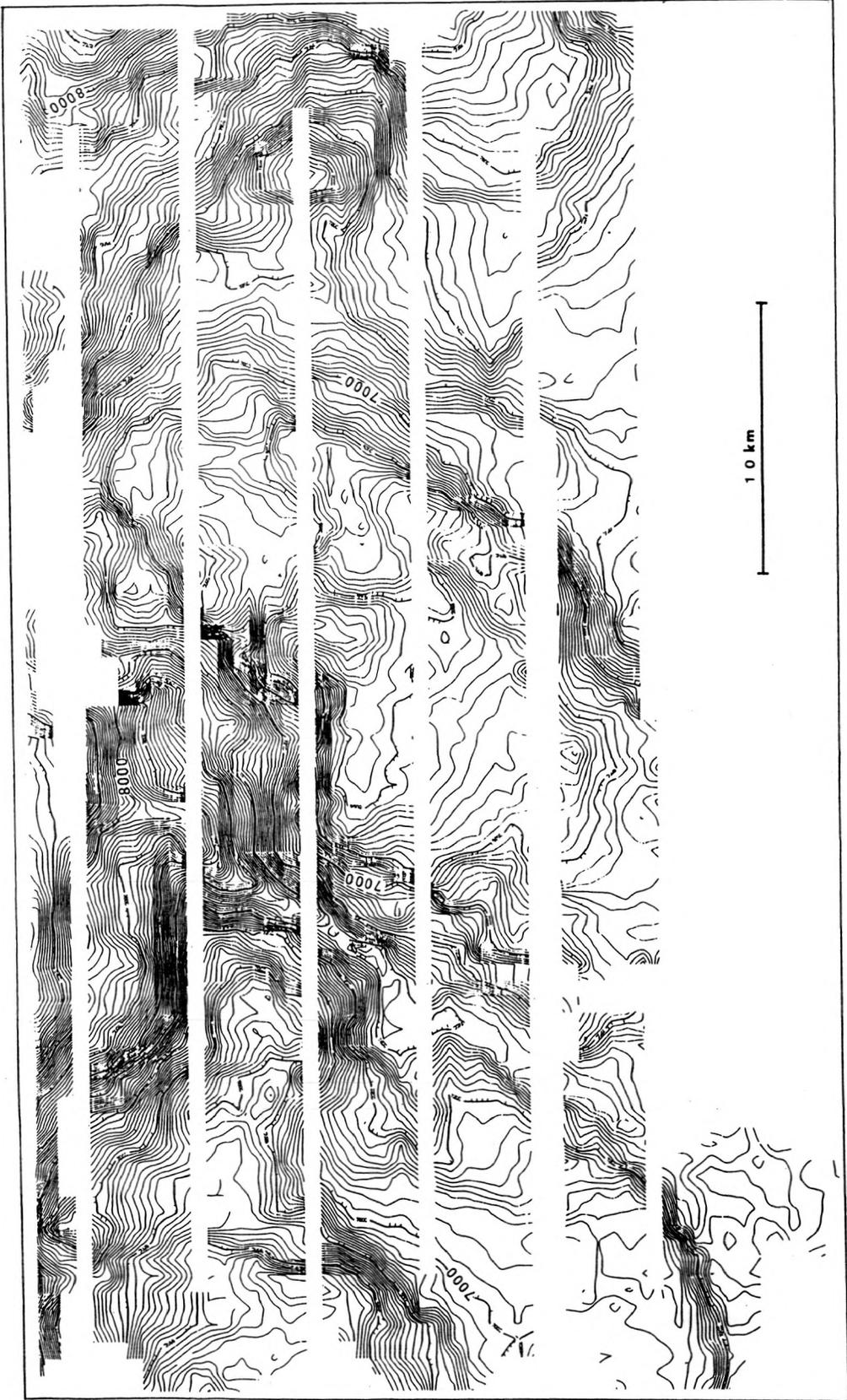
FIG. 3. — Contour chart produced by the on-board contouring program. Contour interval 20 m.
