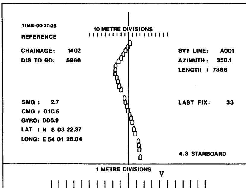
FIG. 4. — Left/Right Indicator Display.
