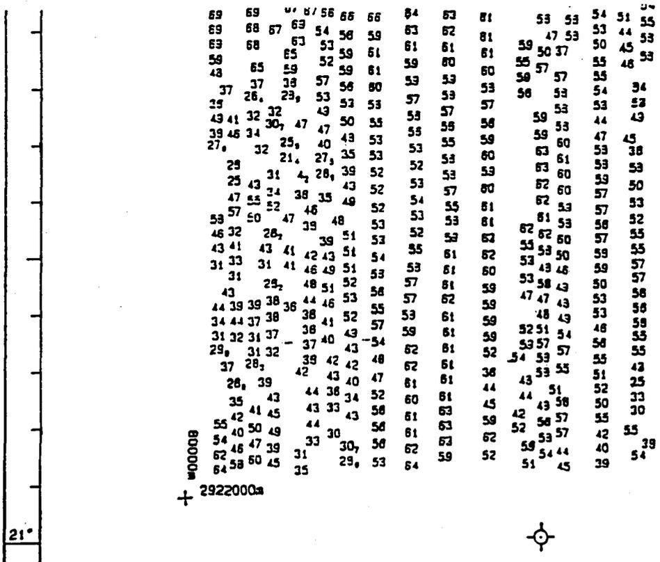
FIG. 7. — Automatically Plotted Survey Fair Sheet.
