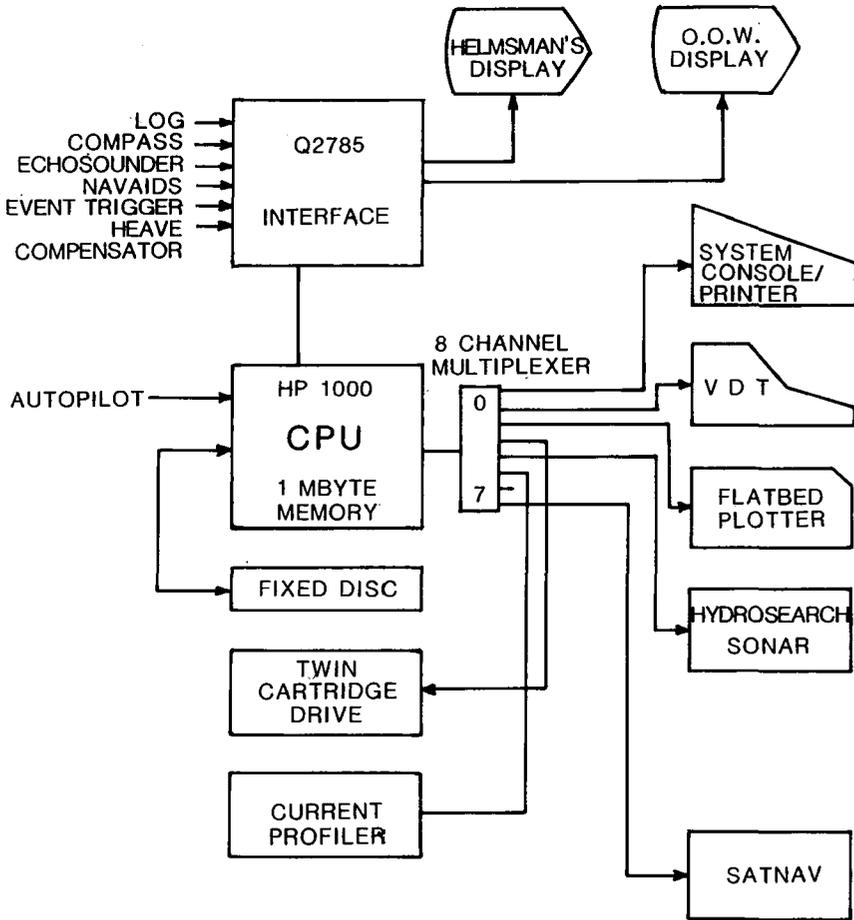
FIG. 2. — Data Logging System (DLS).
