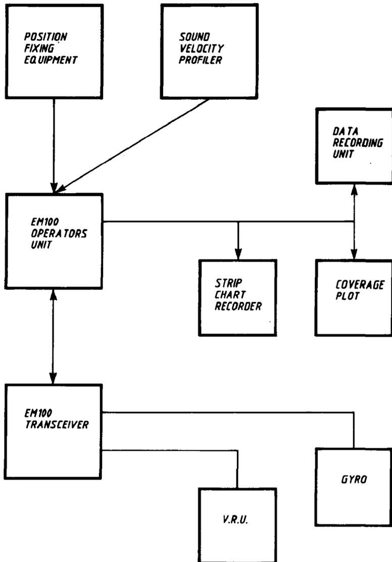
FIG. 2. — Survey ship installation of EM100.
