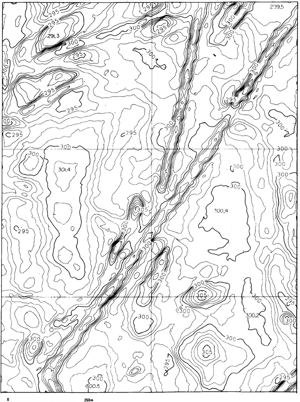
FIG. 7. — Sea floor bathymetry showing iceberg scours and pockmarks. Contour interval 1 metre. Surveyed by A.S. Geoconsult using Simrad EM100.
