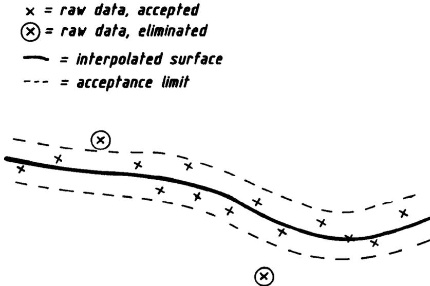
FIG. 6. — Smoothing of data and elimination of noisy data.
