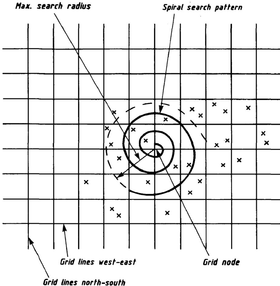
FIG. 5. — Process of going from random data to grid representation.
