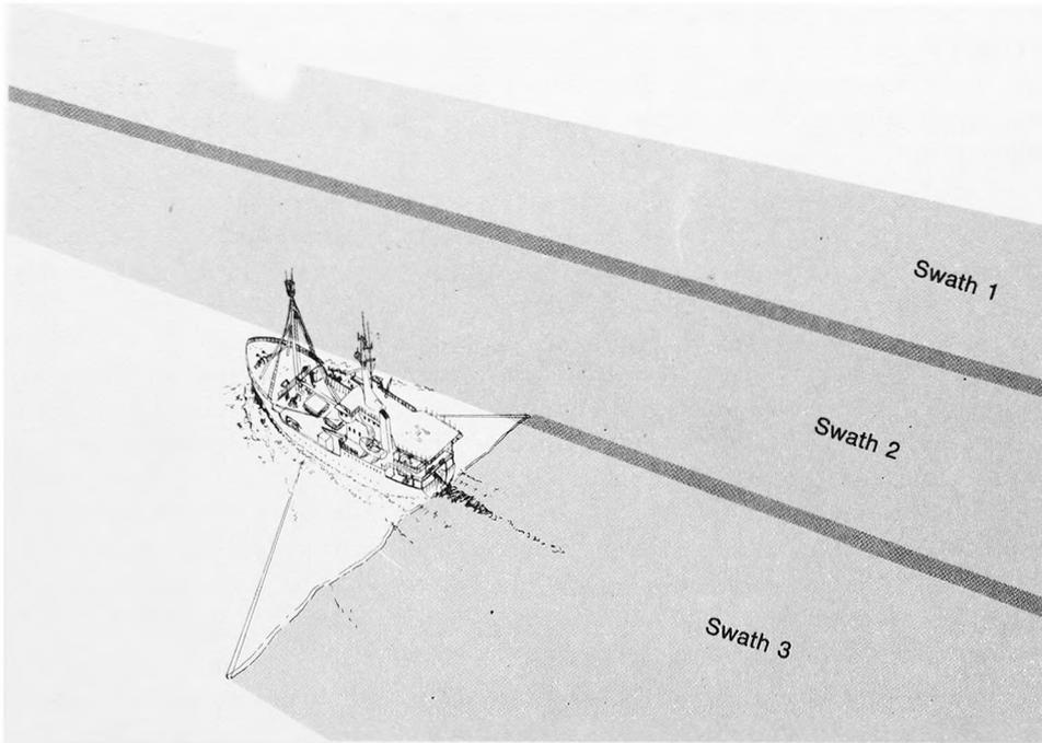
FIG. 13. — Survey method of overlapping swaths.
