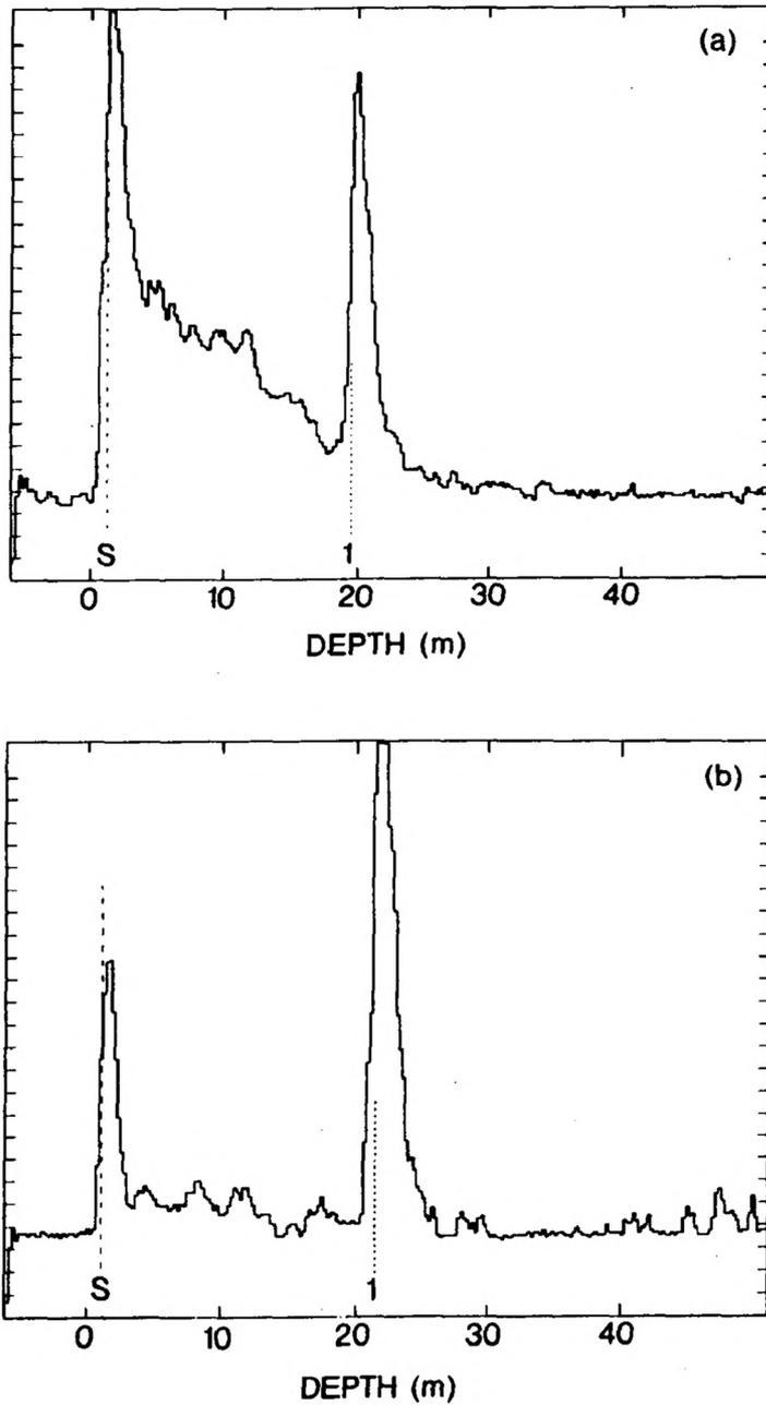
FIG. 8. — Typical WRELADS waveforms, (a) with constant gain across the waveform, and (b) with dynamic photomultiplier gain control in use.
