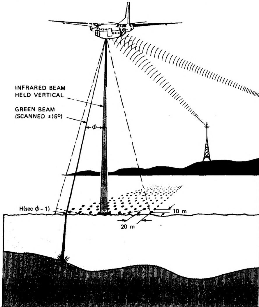
FIG. 1. — Operating scenario for WRELADS laser airborne depth sounder.
