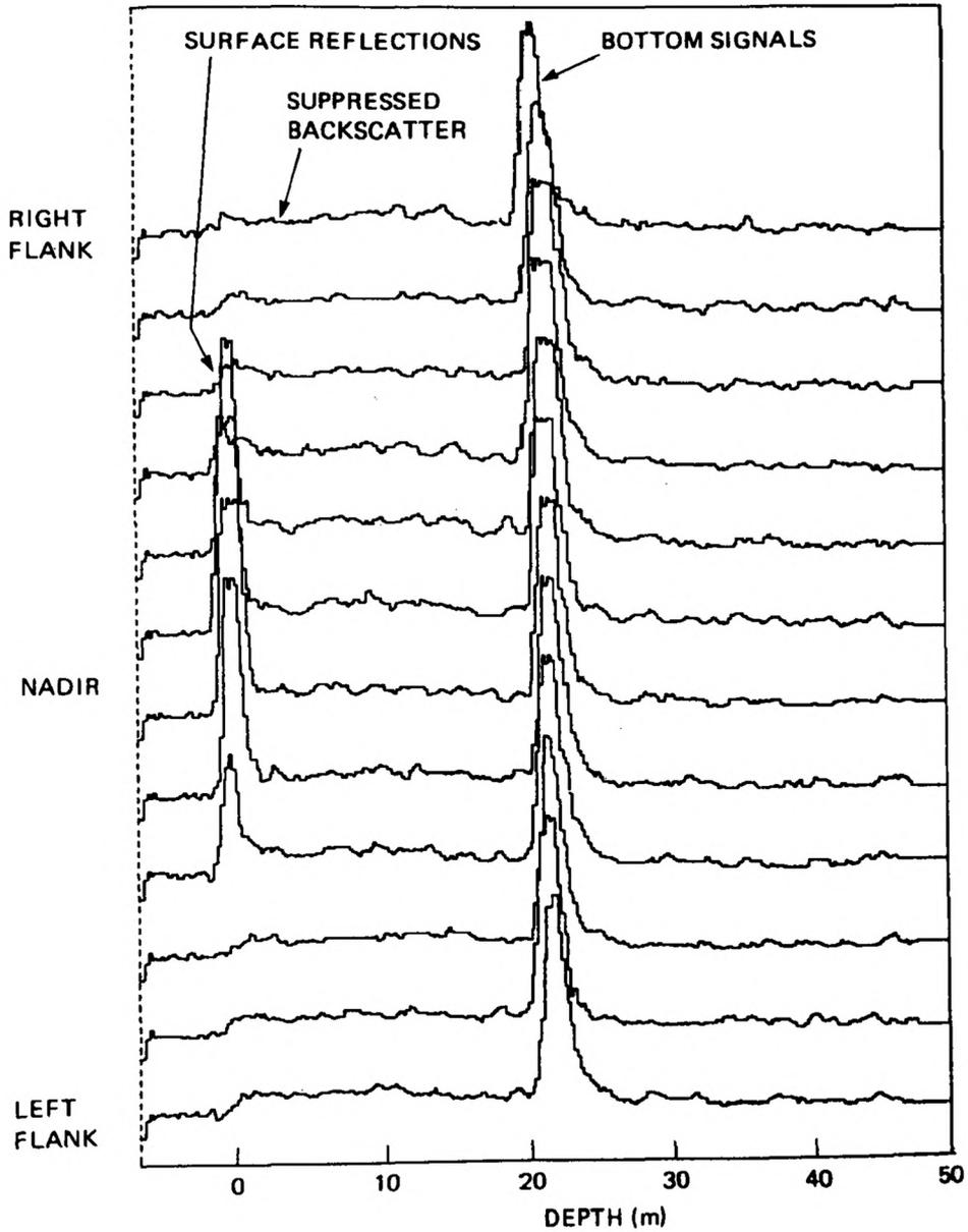
FIG. 3. — Twelve successive waveforms from green laser pulses across a single sweep of WRELADS, with photomultiplier gain control in operation.
