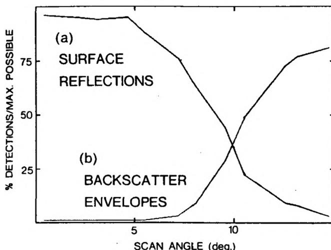
FIG. 9. — Frequency of detection of (a) sea surface reflections, and (b) backscatter envelopes, expressed as a percentage of possible detections, and as a function of scan angle. Each plot represents accumulation of data over 60 sec from the same geographic location, with overflights 40 min apart.
