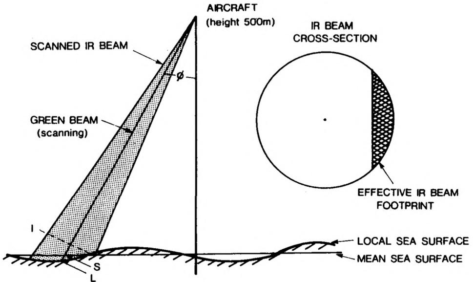
FIG. 7. — Geometry for scanned IR beam with wide divergence.
