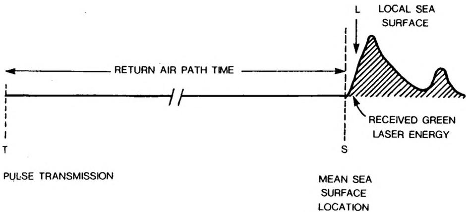
FIG. 4. — Components of received energy offset in time from laser pulse transmission.
