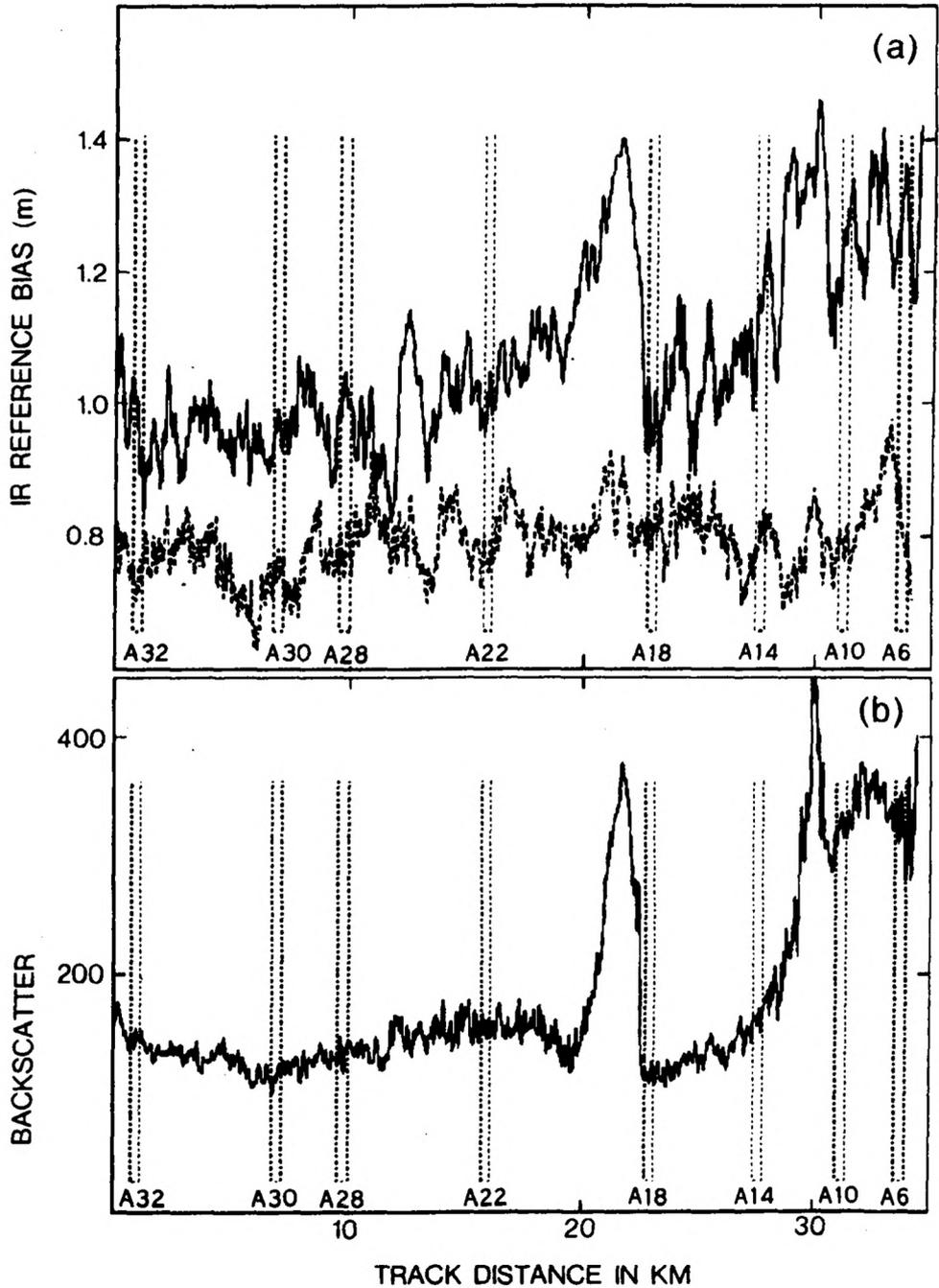
FIG. 10. — Comparison of IR reference bias (IS in Fig. 5) over the same section of sea using first backscatter envelopes only (solid line), and second, surface reflections only (broken line). (b) shows the variation in backscatter amplitude over the same section of sea. The vertical markers show the location of benchmark survey sites.
