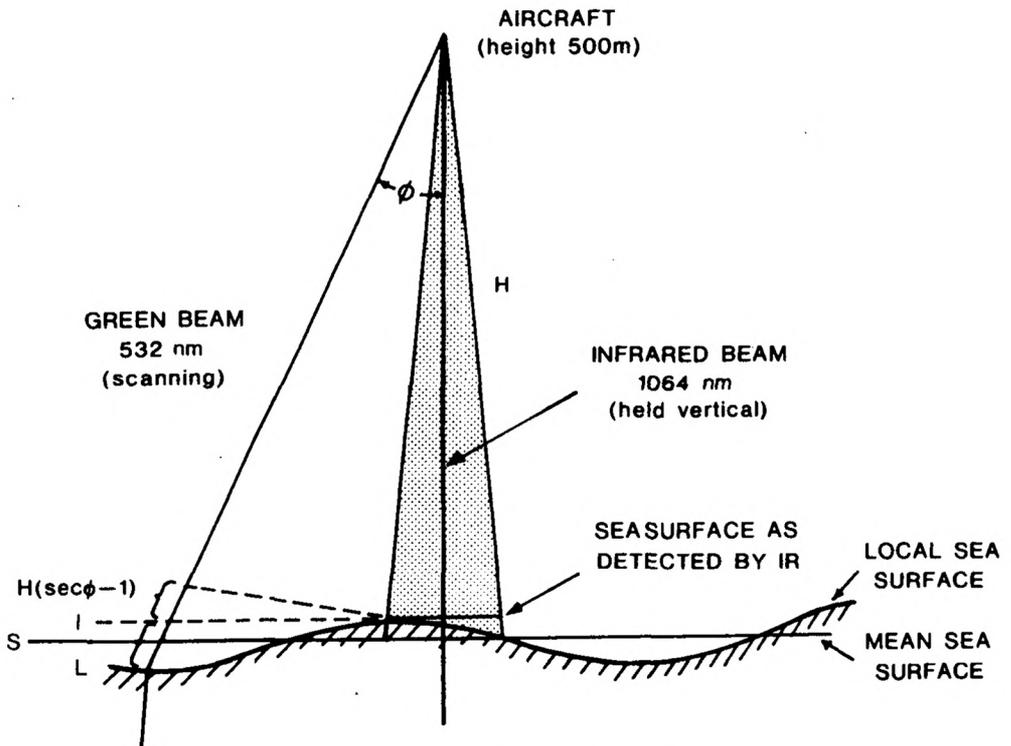
FIG. 6. — Scanning geometry for WRELADS and LADS.
