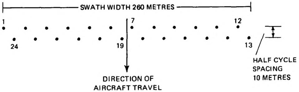
FIG. 2. — Rectangular pattern of green laser spots on the surface of the sea from a single cycle of the WRELADS scanning system.
