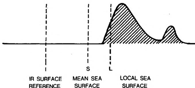
FIG. 5. — Components of received energy offset in time from the new reference point I, which locates the point of IR beam detection of the sea surface (within a constant offset).
