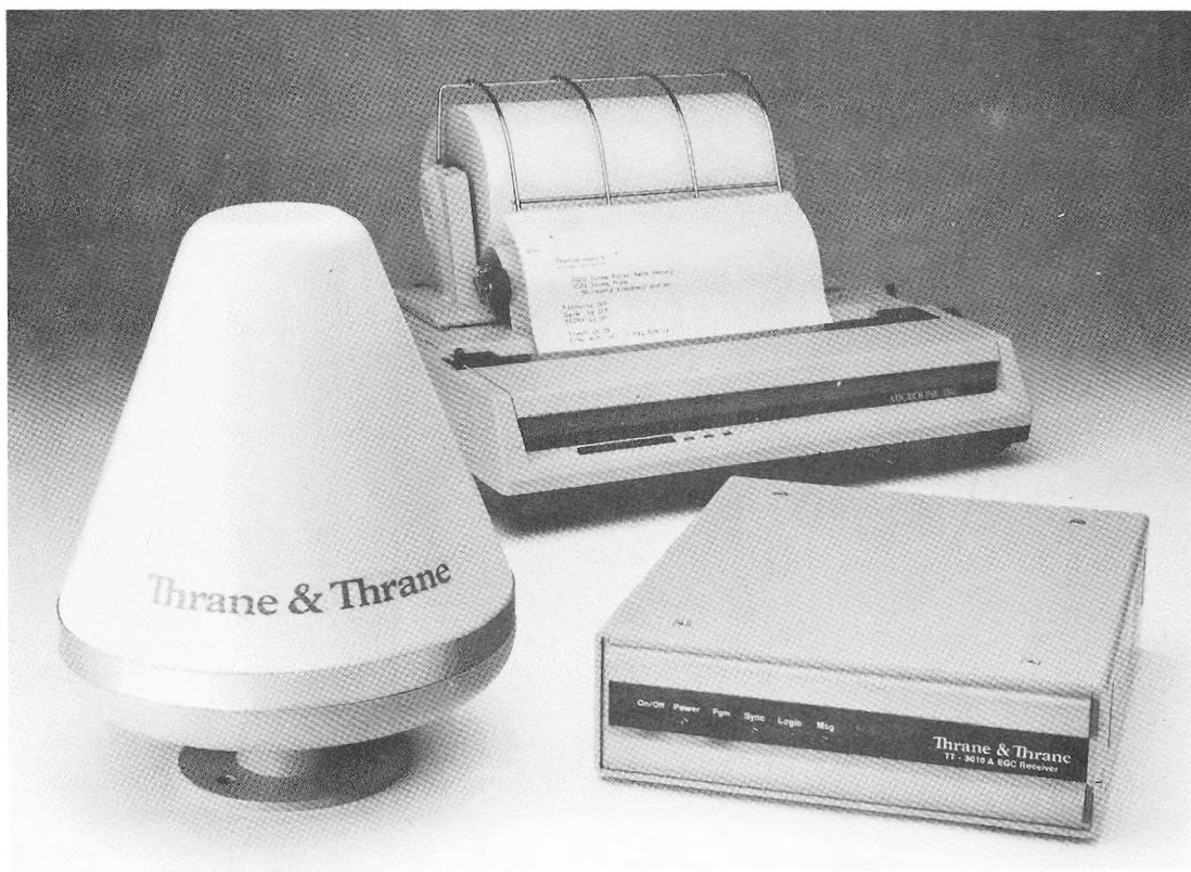
FIG. 10. — EGC Sea Trials receiver and antenna (T & T equipment photo).
