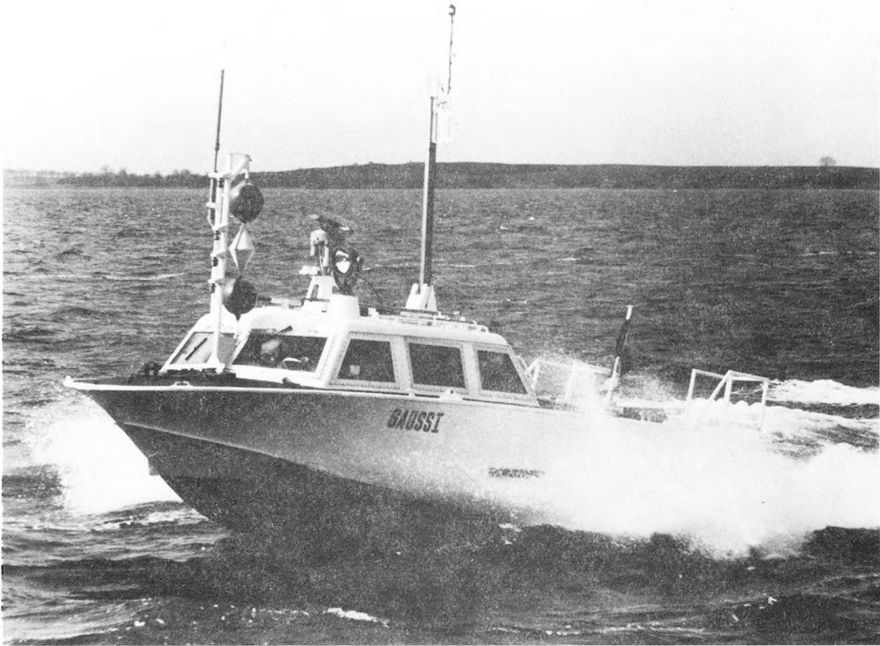
FIG. 3.— The Survey Launch Gauss I . Length overall: 9.85 m; Breadth overall: 3.20 m; v_{\max} : 26 knots; v_{\text{surv}} : 8 knots.
