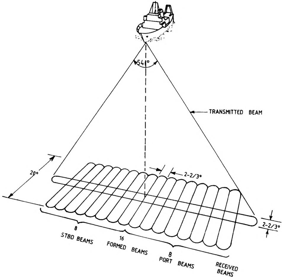
FIG. 4.— Sea beam pattern geometry.
