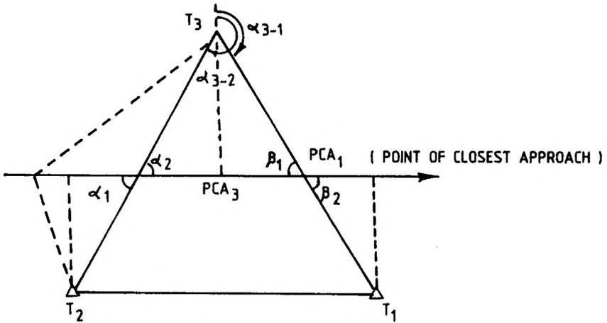
FIG. 2.— Determination of Geometry of Transponders by acoustic line crossing (Moured, 1977).
