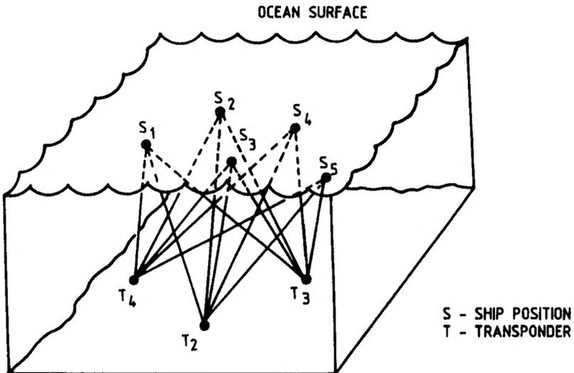
FIG. 3.— Principle of Intersection in Transponder location by surface position (Moured, 1977).
