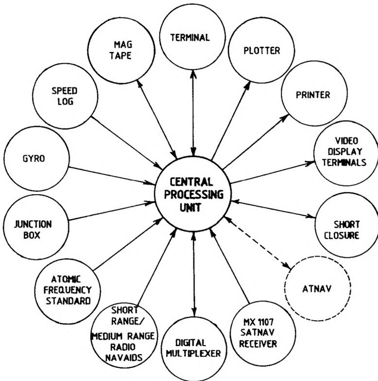
FIG. 1.— Network of Integrated Navigation System.
