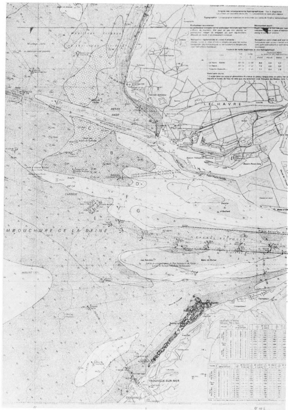
FIG. 4.- Extract from the sediment chart of Le Havre (6736 G) (A: Rock; B: Pebbly gravel; C: Fine gravel; D: Sands; E: Fine sands; F: Clay sands; G: Muds).
