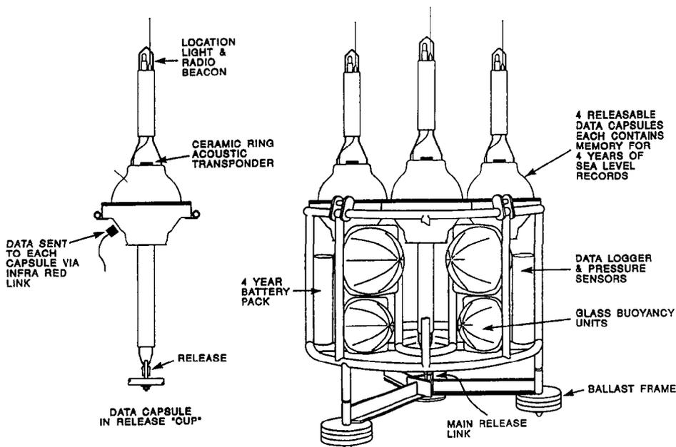
FIG. 6.- Schematic diagram of the Mark 5 long term deep sea pressure recording system with four recoverable data capsules. This initial system will be capable of recording data for five years in the deep ocean with data capsule recovery each year.
