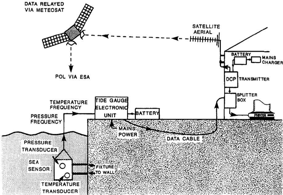
FIG. 5.- Schematic of the ACCLAIM coastal gauge showing the pressure and temperature sensors and tide gauge electronics, including the Data Collection Platform (DCP) which communicates with the Meteosat satellite. Data from the European Space Agency (ESA) are sent to POL via telex.
