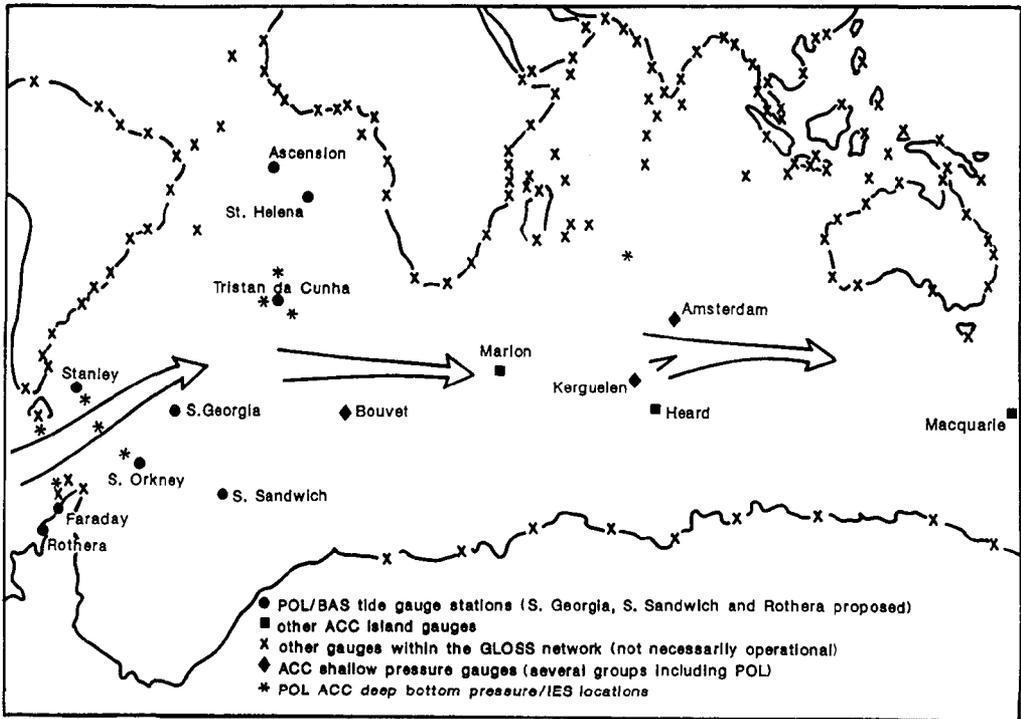
Fig. 1.- Map showing the locations of ACCLAIM sea level and bottom pressure stations and those of collaborating organisations. The use of recorders in pairs to monitor changes in ACC flow is shown schematically.
