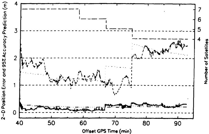
FIG. 4.- HPM/NovAtel Static Position Accuracy Test
