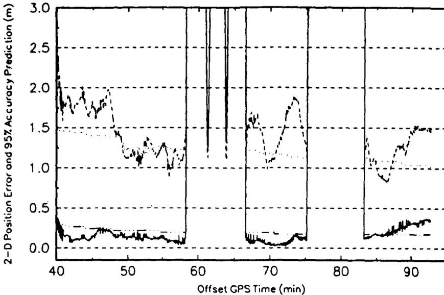
FIG. 5.- HPM/Novatel Static Position Accuracy Test
