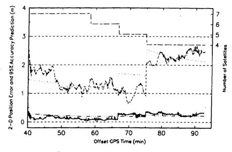
FIG. 4.- HPM/NovAtel Static Position Accuracy Test A Priori and Measured Accuracies in Reduced Coverage.
