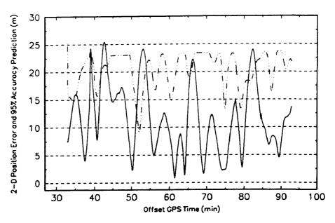
FIG. 6.- HPM/Novatel Static Position Accuracy Test Single Point Statistics Using NovAtel measured Range Accuracies.
