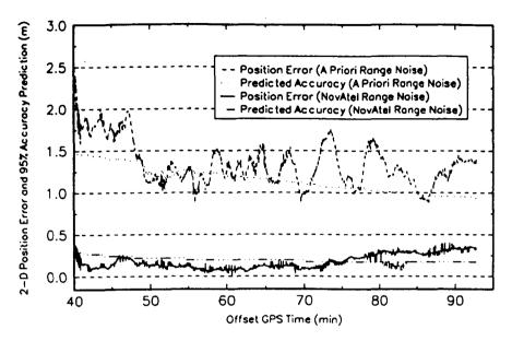
FIG. 3.- HPM/NavAtel Static Position Accuracy Test Using a Priori and NovAtel Measured Range Accuracies.
