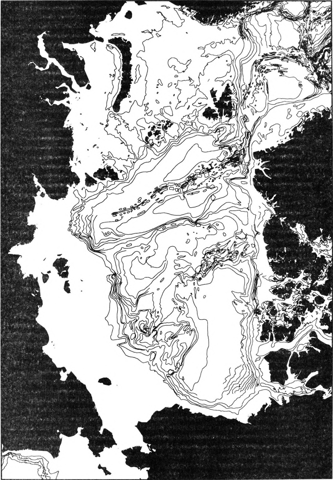
FIG. 5.- Arctic bathymetric contours extracted from the GEBCO Digital Atlas (GDA). Drawn originally by hand for the Fifth Edition of the General Bathymetric Chart of the Oceans, these contours were digitized recently and placed into public circulation in a computer-readable form. For clarity, this figure does not illustrate all the information north of 64°N that was extracted from the GDA for the purposes of this study; contours are shown at 200-metre intervals only, while areas such as Baffin Bay, the Canadian Arctic Archipelago, and the Norwegian-Greenland Sea, are only partially or not shown.
