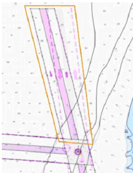
Figure 5 – Misalignment of two Traffic Separation Scheme (TSS) objects
