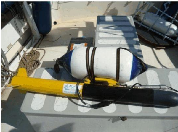
Figure 10. Investigation of optimum ultra shallow water deployment technique for sidescan towfish.
