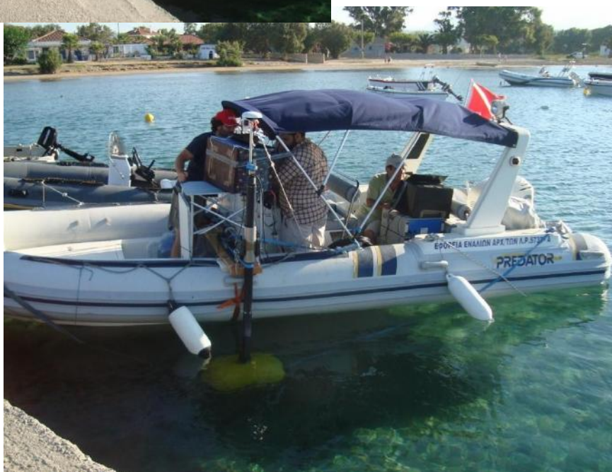
Figure 16. System checks of the GeoAcoustics GeoPulse Pinger.
