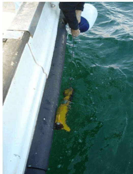
Figure 10. Investigation of optimum ultra shallow water deployment technique for sidescan towfish.
