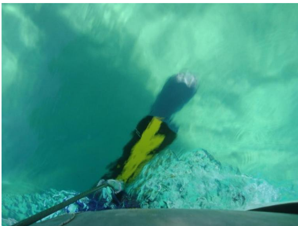
Figure 14. The GeoAcoustics sidescan sonar towfish deployed by the bow of the survey boat.
