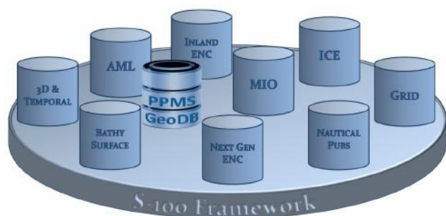
Figure 2 - S-100 framework with PPMS GeoDB among some other future S-100 series products. Developing within the S-100 framework allows the GeoDB to adopt already developed resources (simplifying implementation) and present its data in a common framework (simplifying adoption).
