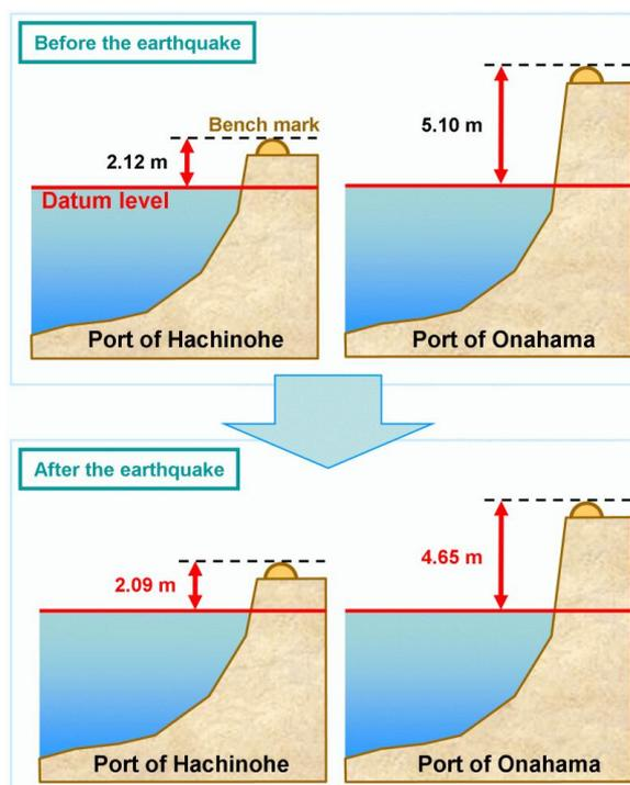
**Figure 14** Land subsidence found in determination of a datum level at Ports of Onahama (right panel) and Hachinohe (left panel).
