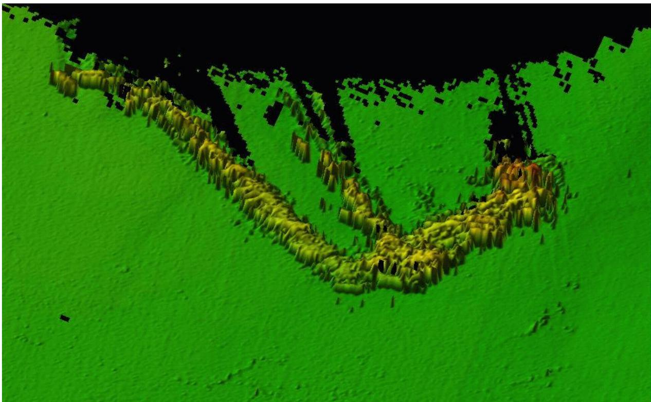
**Figure 8** The multibeam echo sounder record of a fallen crane from a quay.
