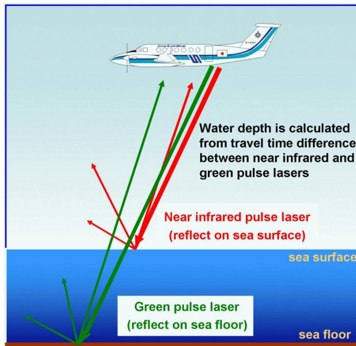
**Figure 11** The principle of airborne LIDAR bathymetry.
