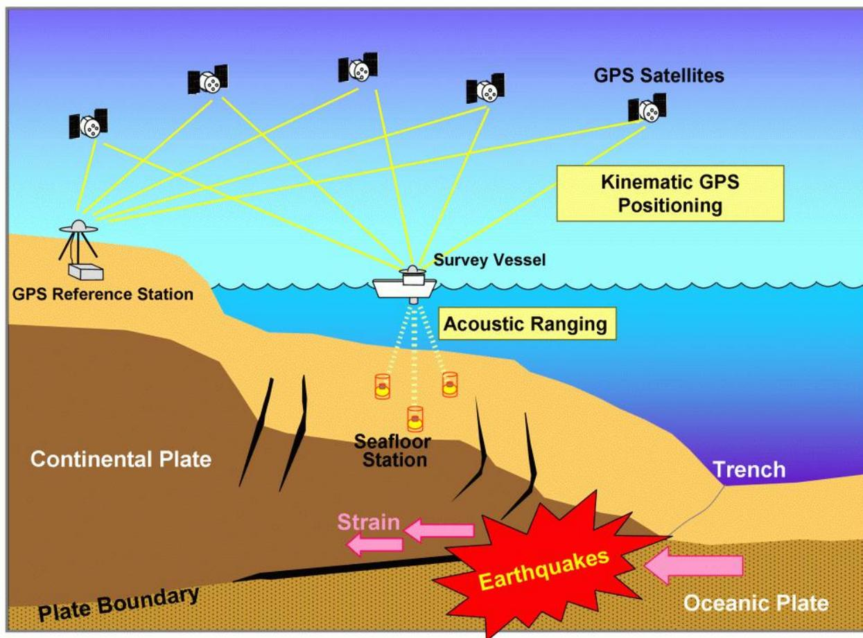
**Figure 9** The GPS/acoustic combined method of seafloor geodetic observation
