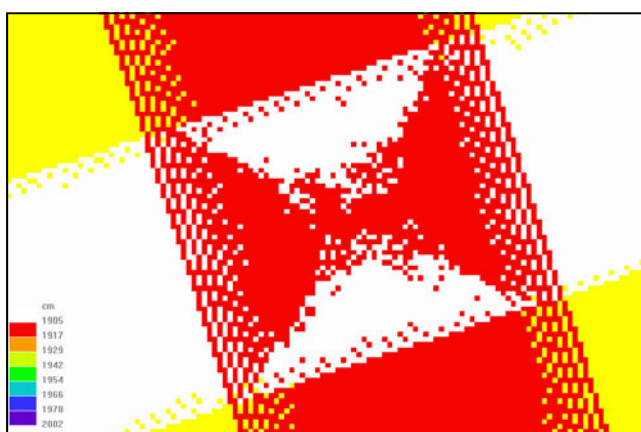
Figure 1. Distribution of cells in DTM of survey track (red) and check line (white).
