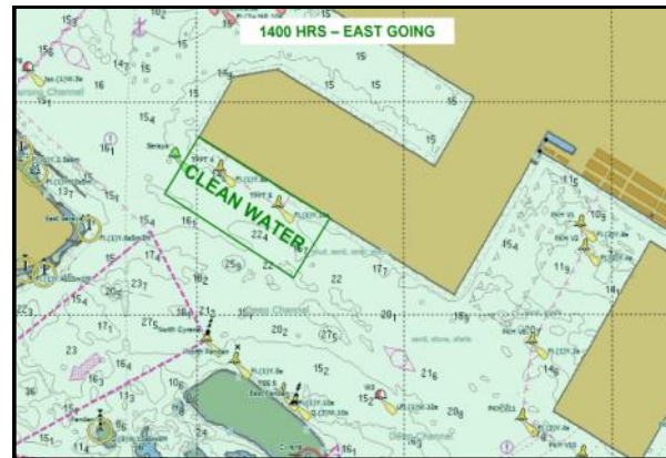
Sample Display on a “green” ECDIS of Designated Area for Ballast Water intake shown at 1400 to 1500 hrs. Size of area changed due to tidal flow
