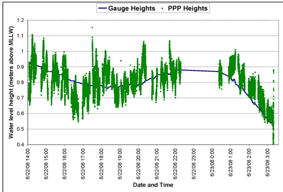
Figure 12: PPP water level height versus tide gauge water-level height
