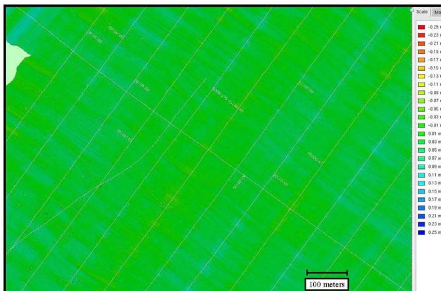
Figure 7: Difference grid produced by subtracting PPK vertical-controlled CUBE surface from tide-gauge-controlled CUBE surface
