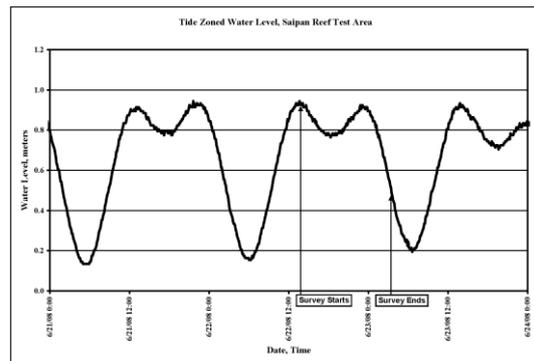
Figure 2. Water level heights relative to MLLW, showing variation over time frame of survey
