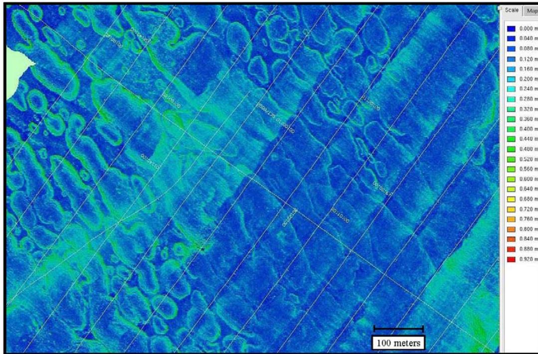
Figure 8: CUBE standard deviation for PPP vertical-controlled depth
