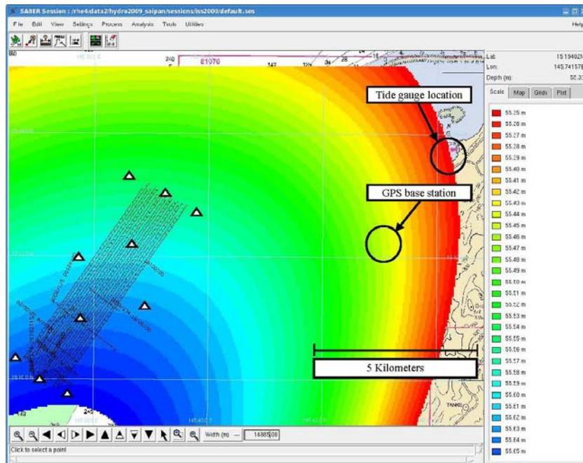
*Figure 5: EGM 2008 model of geoid undulation over the survey area*
