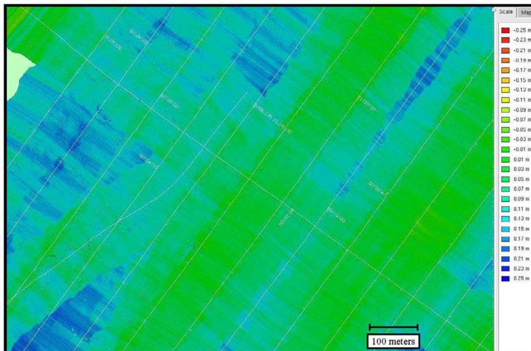
Figure 9: Difference grid produced by subtracting PPP vertical-controlled CUBE surface from tide-gauge-controlled CUBE surface
