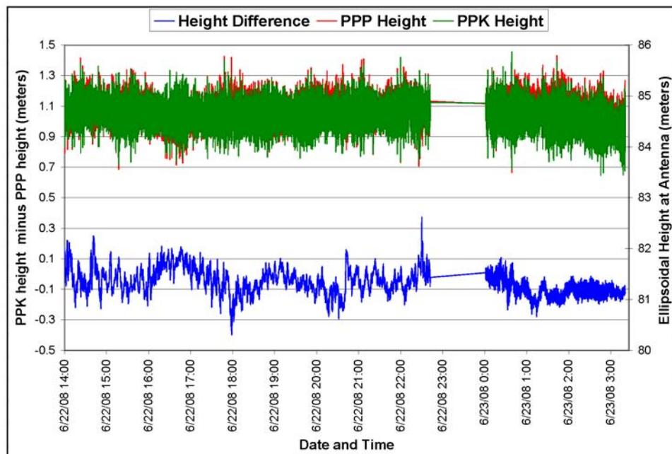
Figure 13: Comparison of PPP height solution against PPK height solution
