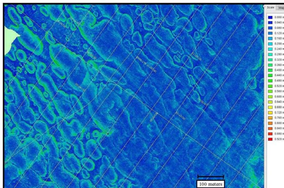
Figure 6: CUBE standard deviation for PPK vertical-controlled depth
