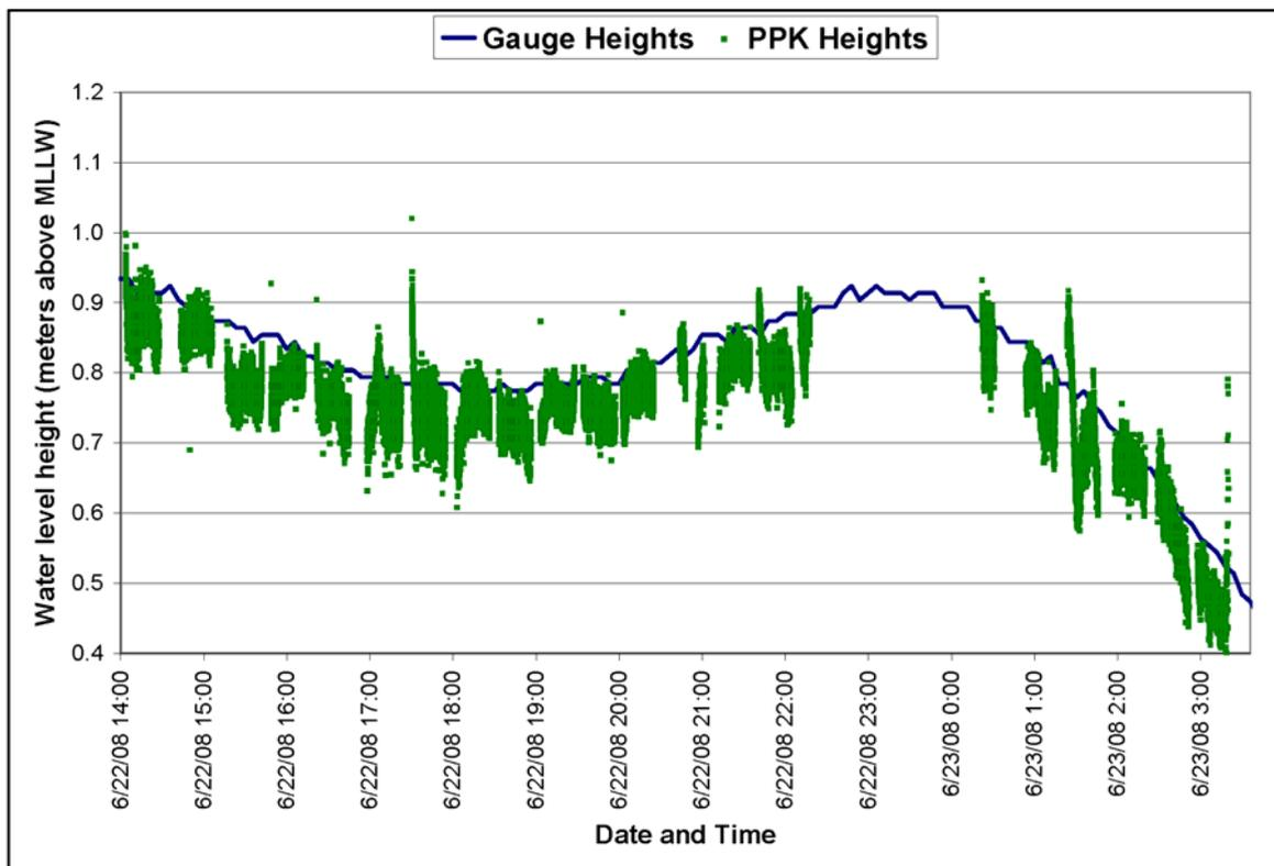
Figure 11: PPK water level height versus tide gauge water-level height
