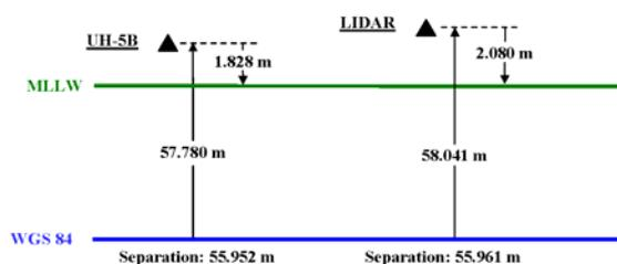
Figure 4. Separation definition at benchmarks in vicinity of installed tide gauge
