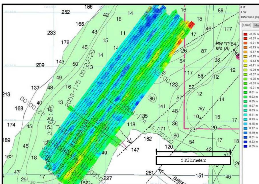
Figure 10: Difference surface produced when PPP vertical-controlled depth is subtracted from tide gauge vertical-controlled depth
