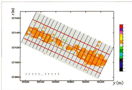
Figure 13: seabed evolution within 2 months in the monitored water area. The blue line denotes transect line and the red line denotes check line.
