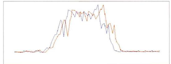
Figure 6: An inconsistency between to-and-fro sounding profiles resulted from time offset. In the figure, the blue and red lines represent two-way profiles respectively.
