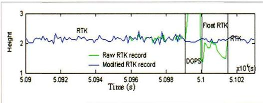
Figure 5: The integrated modification with GPS tidal level and heave. The green line reflects raw GPS height series, while the blue reflects amended one.
