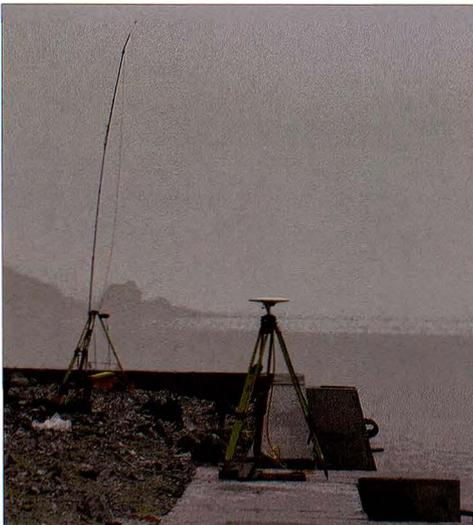
Figure 1: RTK reference station.
