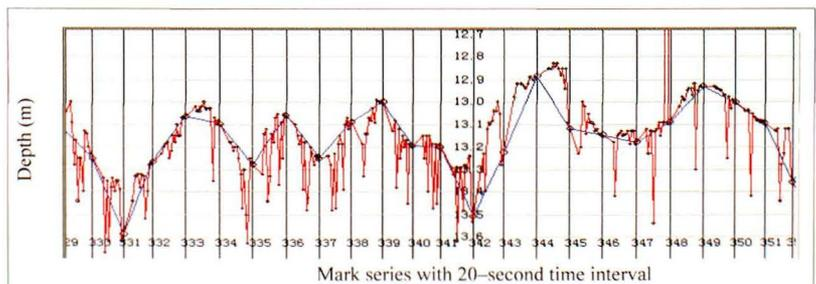
Figure 3: Sounding edit. Red line is echogram with 1-second surveying rate. Blue line denotes actual samples with 20-second sampling rate.
