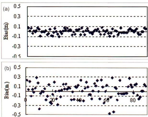
Figure 11: the distribution of height difference at each of the cross point pairs. The tide-independent method is used in (a), while the tide-dependent (traditional) method is used in (b).
