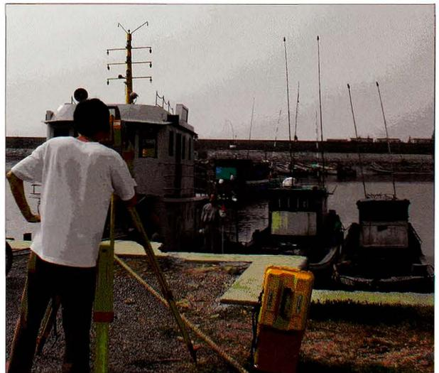
Figure 2: Measuring lever arms of sensors on VFS.
