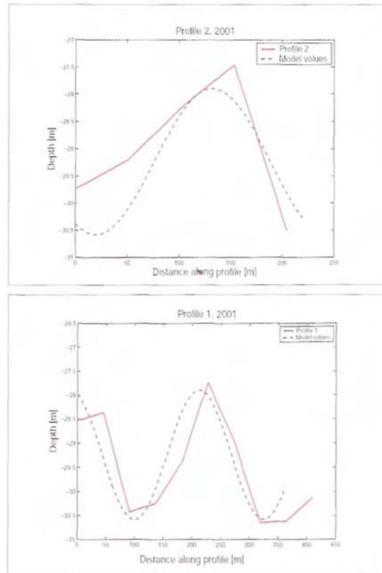
Figure 9: Two profiles of the modeled (blue) and real (red) sand waves. The location of the profiles is indicated in Figure 5.
