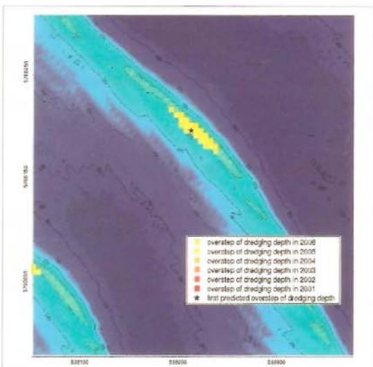
Figure 7: Predicted moments of crossing of the dredging depth as determined by the state-space approach. Coordinates are in UTM31-WGS84.
