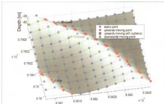
Figure 6: Results of the deformation analysis per node, colour intensity corresponds to size of the trends found. Additionally, values for the maximum trend and the outlier are given. Coordinates are in UTM31-WGS84.
