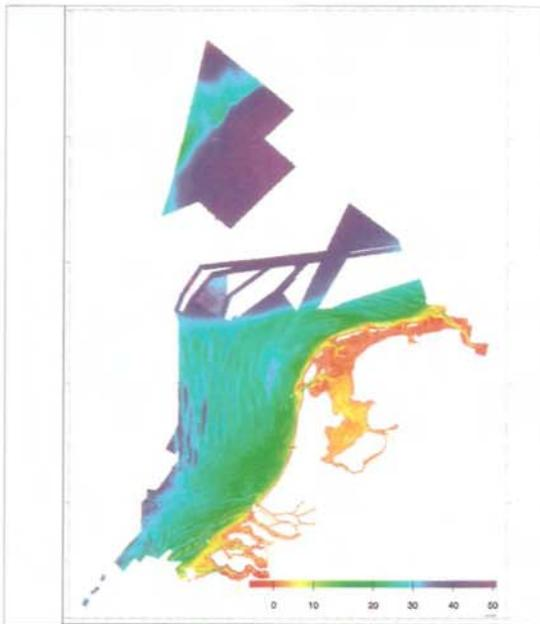
Figure 1: Dutch coastal bathymetry, as stored in the bathymetric archives of the Hydrographic Service. The empty spaces have not yet been resurveyed since the creation of the digital archives.
