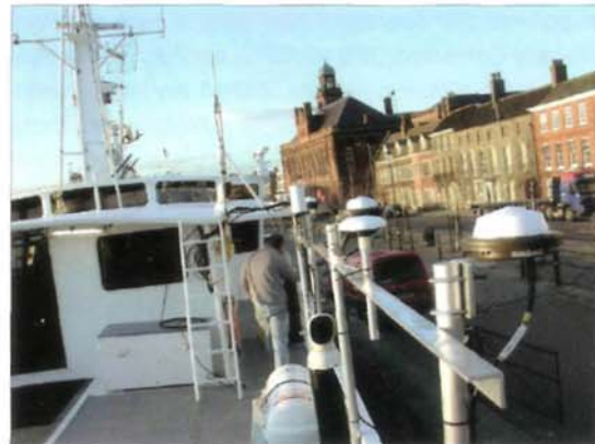
Figure 6: GPS antennae installations onboard MV Confidante.
