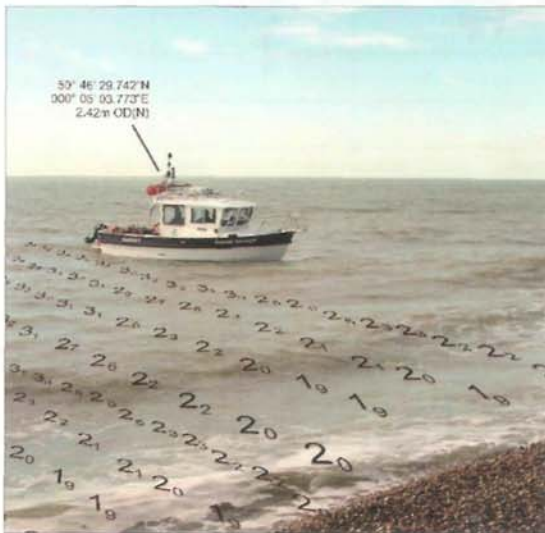
Figure 13: RTK surveying in near-shore area; soundings reduced to land datum (ODN).
