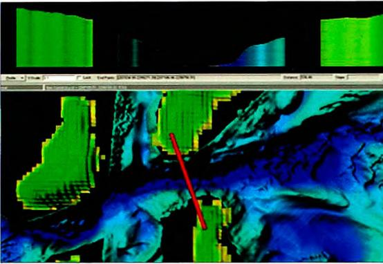
Figure 1: Fusion of altimetric data from BdAlti IGN (green), multibeam survey SHOM (blue) The cross section makes it appear as a large gap between data (black area ~50m large).
