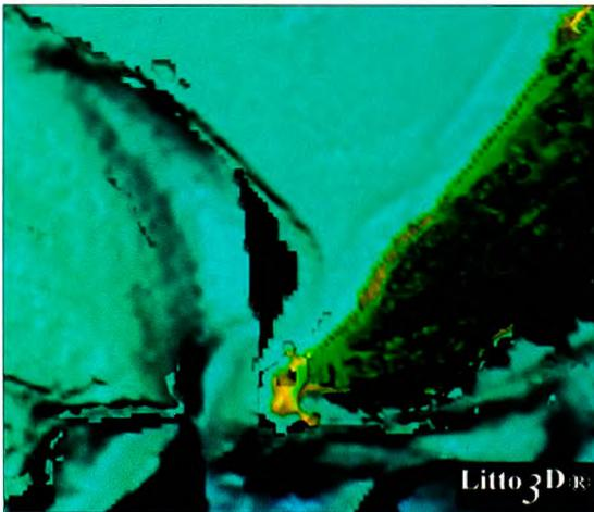
Figure 6: Areas not detected between the bathymetric laser and the MBES survey.
