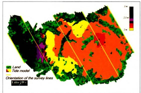
Figure 2: Evolution of tide height along flight tracks (heights in metres).
