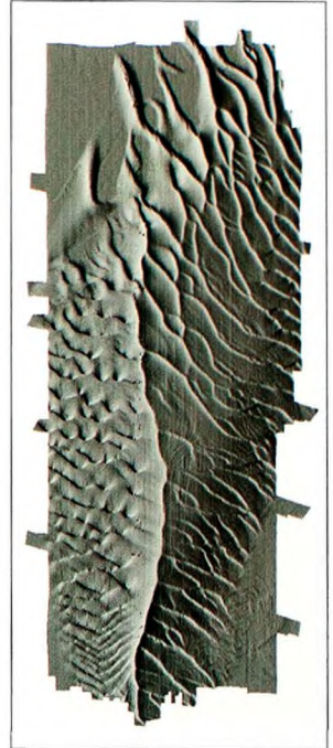
Figure 12: Shaded Terrain digital model based on survey SMF EM1002S on Schôle bank (SHOM, 1999).
