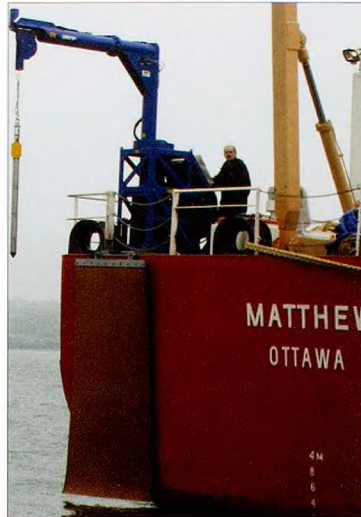
Figure 1. Photograph of the FFCPT and MVP installed on CCGS Matthew in preparation for field trials in November, 2005.
