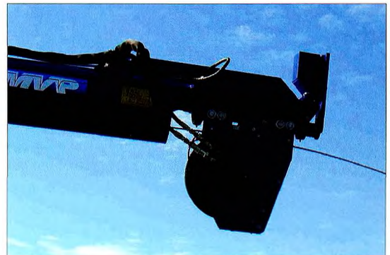
Figure 5. Photograph of the line puller that replaces the normal over-boarding sheave on the MVP to prevent the cable drum from over-rotating when the FFCPT impacts the seabed.
