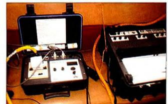
Photo 4: The magnetometer and side scan sonar consoles. (Photo Courtesy: Innocent Egbuh).
