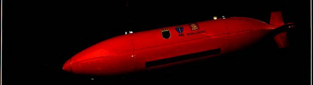
Synthetic aperture sonars combine a number of acoustic pings to form an image with much higher resolution than conventional sonars, typically 10 times higher.
