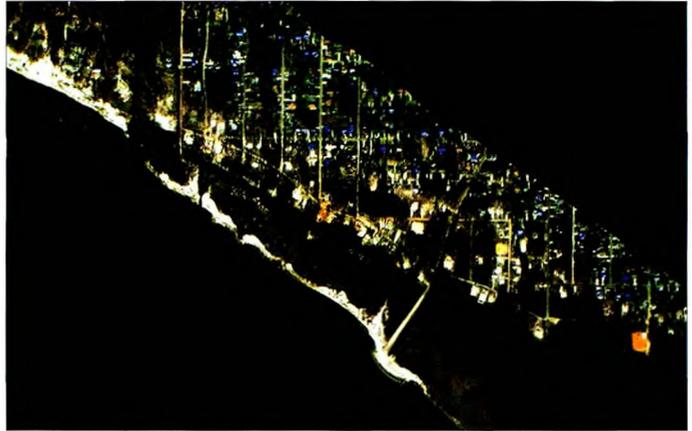
Figure 3: RGB extracted from 36 bands of CASI-1500 hyperspectral data collected near Ocean Springs, Mississippi, following Hurricane Katrina. Areas where there are houses, but no FEMA blue roofs, are areas where storm surge inundated the coast and either destroyed homes completely or made them unlivable.
