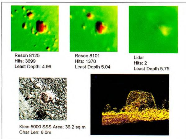
Figure 8: Example 2. This object was detected, but the least depth was not accurate to IHO order 1.
