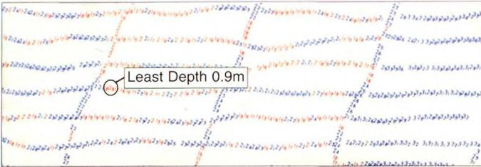
Figure 9 - Acoustic survey across boulder bed.
