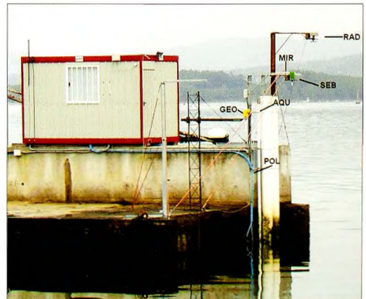
Figure 2: Test station with the tide gauges that formed part of the experiment and the hut where the electronic devices were kept. In the photograph we can see the horn-antenna of RAD, SEB and GEO radars, the planar antenna of MIR radar, the protection tube of the AQU acoustic gauge, and the submerged POL gauge.
