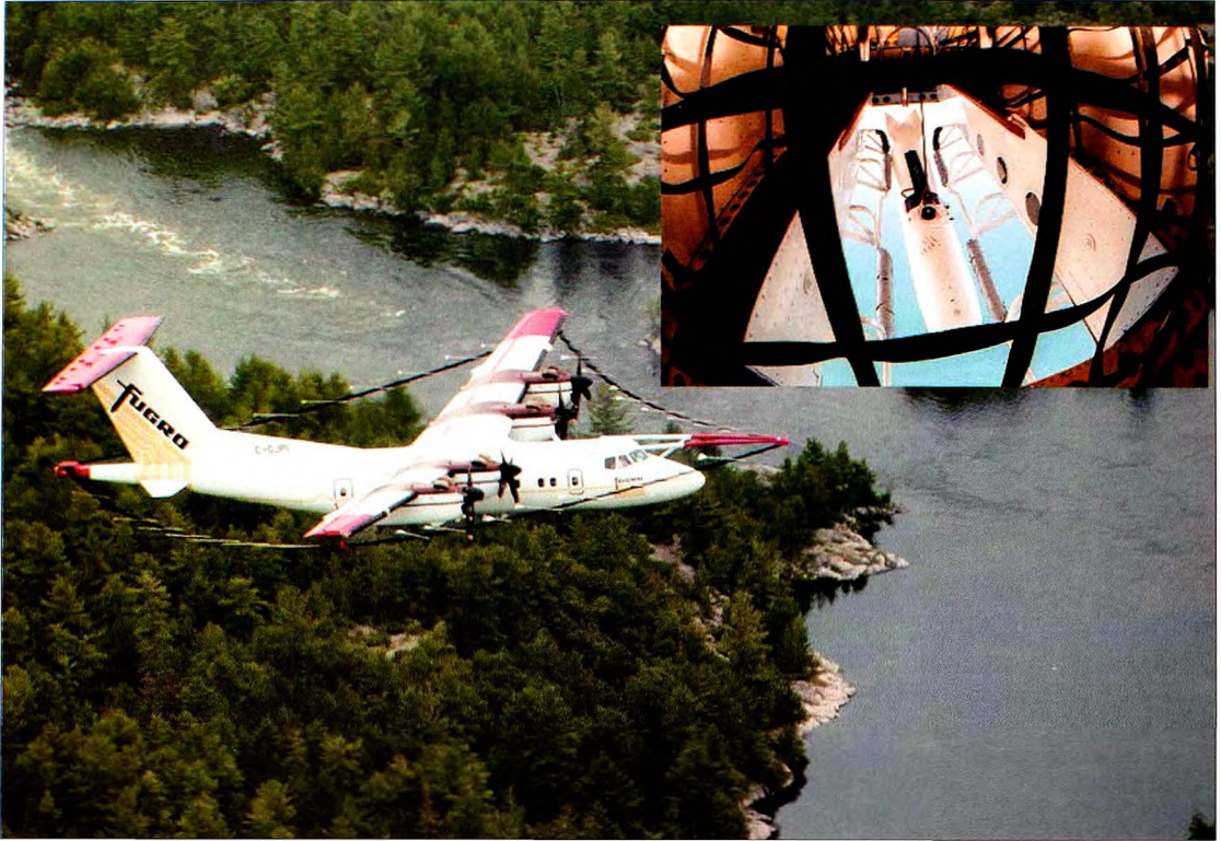
Figure 5: GEOTEM AEM system and an AEM bird deployment (inset).
