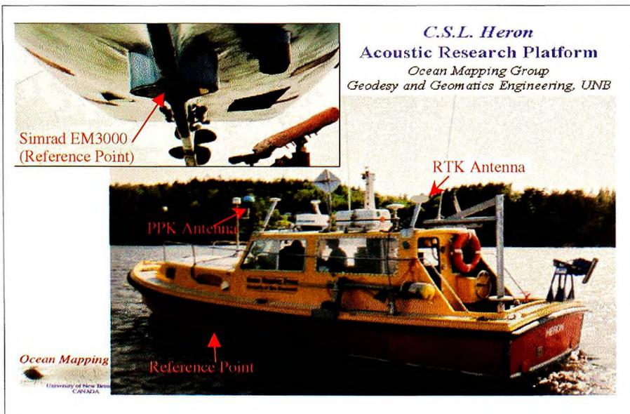
Figure 3: The locations of the two GPS rover antennae on the *HERON*.
