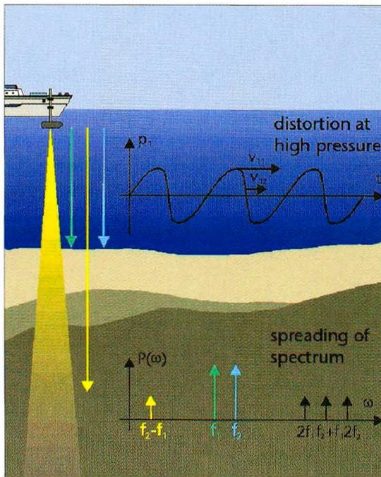
Figure 1: The principle of parametric acoustics
