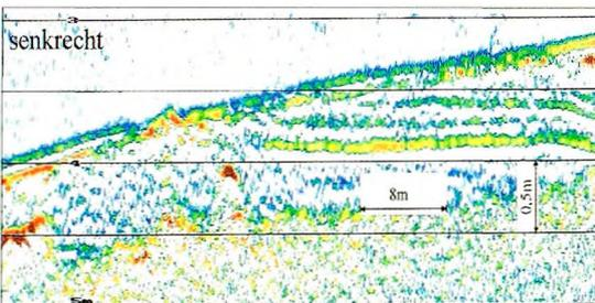
Figure 17: Echoprint from a Viking barrier (vertical beam)
