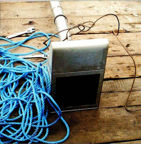
Figure 4: Parametric transducer
