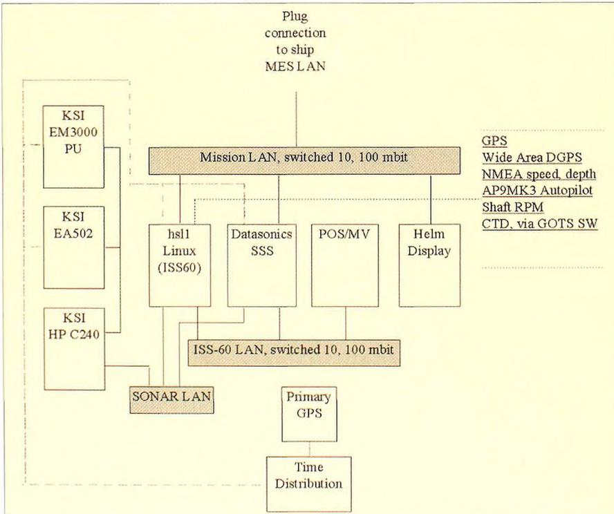
Figure 3: High-level ISS-60 and Mission Electronics Suite (MES) block diagram for HSL configuration
