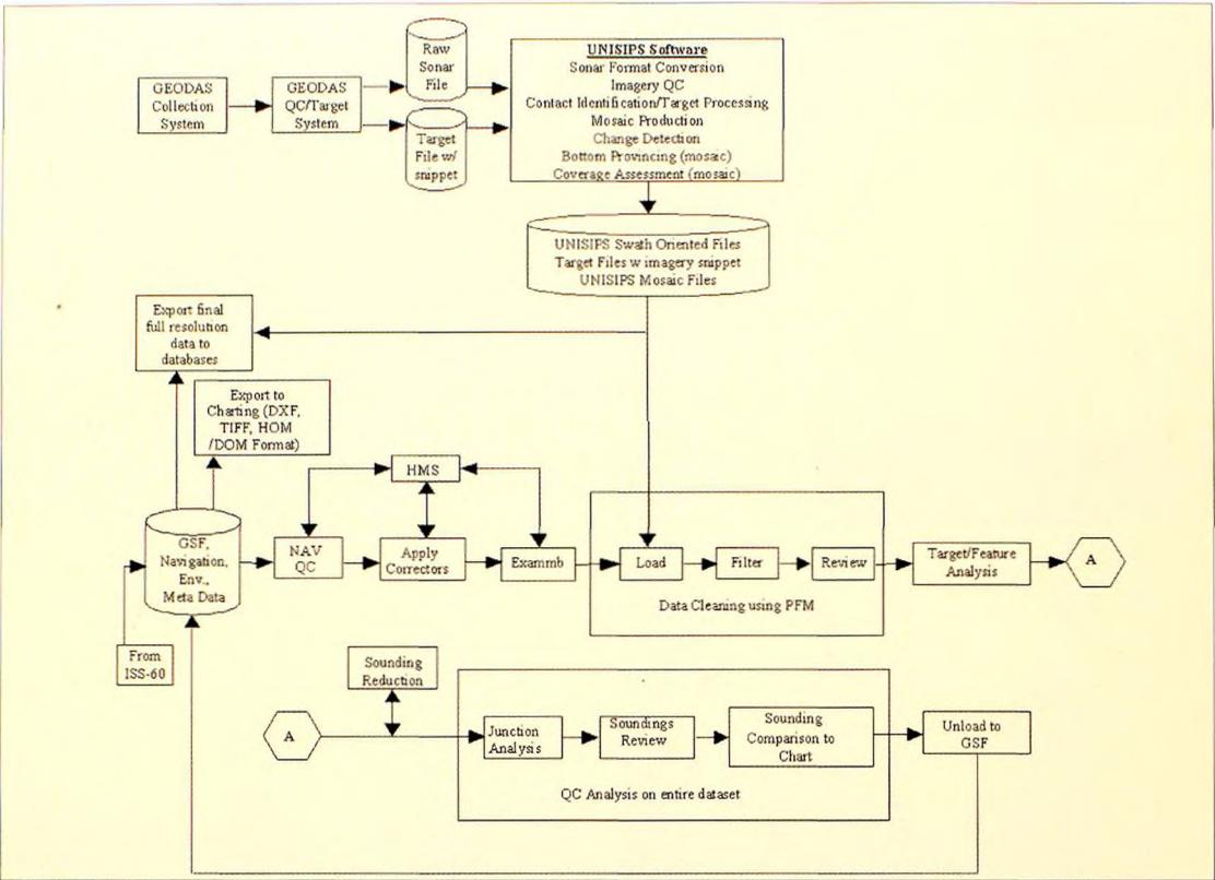
Figure 11: NAVOCEANO Shipboard Hydrographic / Processing Pipeline
