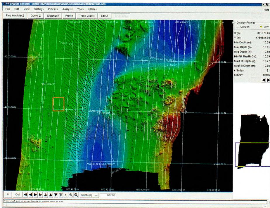
Figure 13: Reson 8125 data from Portsmouth, N.H. 0.5 metre PFM, minimum filtered depth surface coloured by depth
