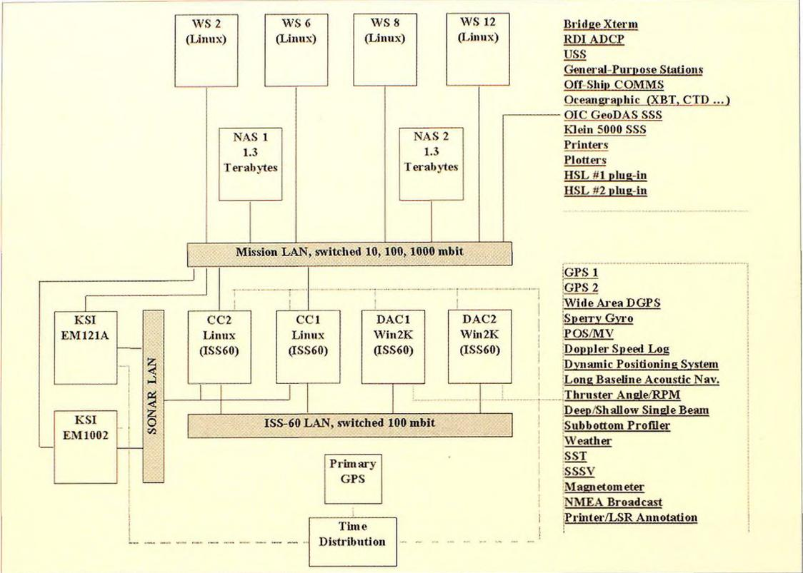
Figure 2: ISS-60 and Mission Electronics Suite (MES) block diagram for T-AGS 60 class ship configuration
