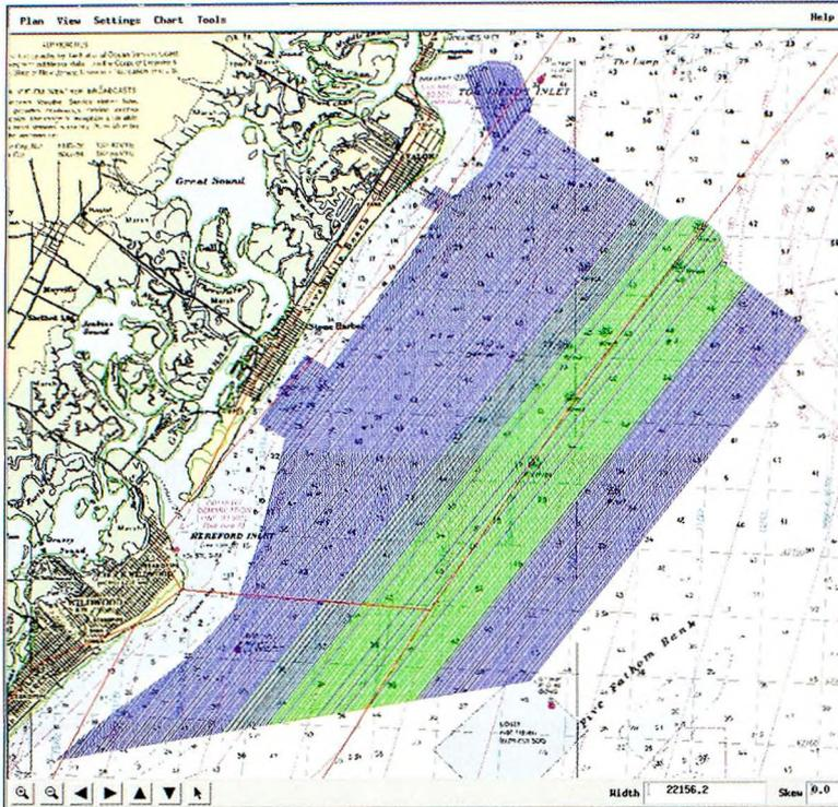
Figure 5: Survey lines planned over chart (Green indicates the line has been run)
