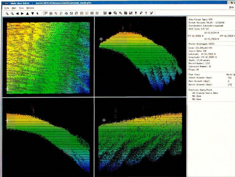
Figure 15: Multi-view interactive editor showing all contributing soundings selected from a subset of the PFM file
