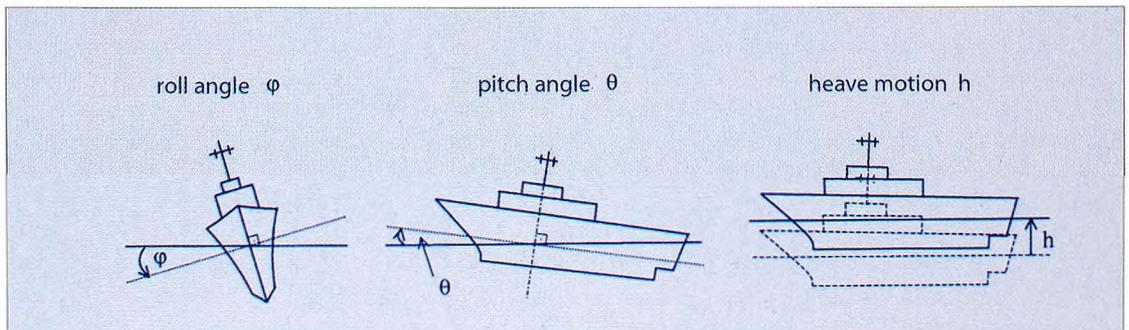
Figure 4.2: Schematical demonstration of marine motions. The definition of the analysed motion parameters roll (left), pitch (middle), and heave (right) are illustrated, the arrows indicate the direction of increasing values
