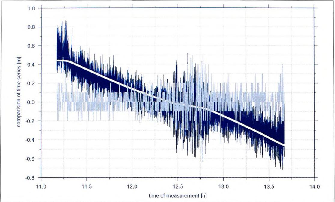
Figure 9.1: Results of the vertical motion in comparison. The GPS solution (black line) and the heave recorded by the INS sensor (grey line) are shown for the same time section. The GPS-derived heights are centred to the averaged INS value. The impact of the geoid height on the GPS solutions (white line) is centred to the mean value, too
