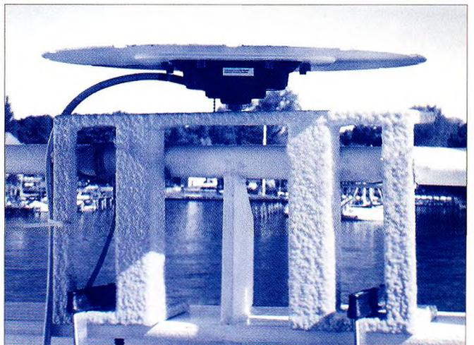
Figure 3: Example of the mounting of a GPS antenna on the *DENE B* (top deck)
