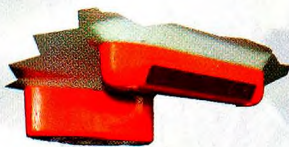
Actual transducer installation with a 38/200 kHz and a side- looking sonar transducer
