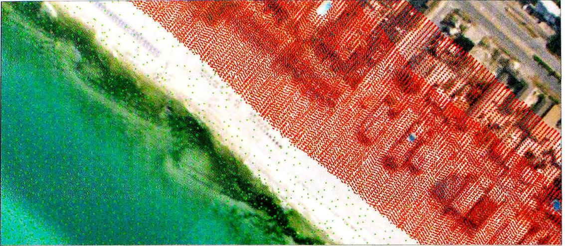
Figure 1a: Fusion of hydrographic and topographic lidar data with imagery: data points
