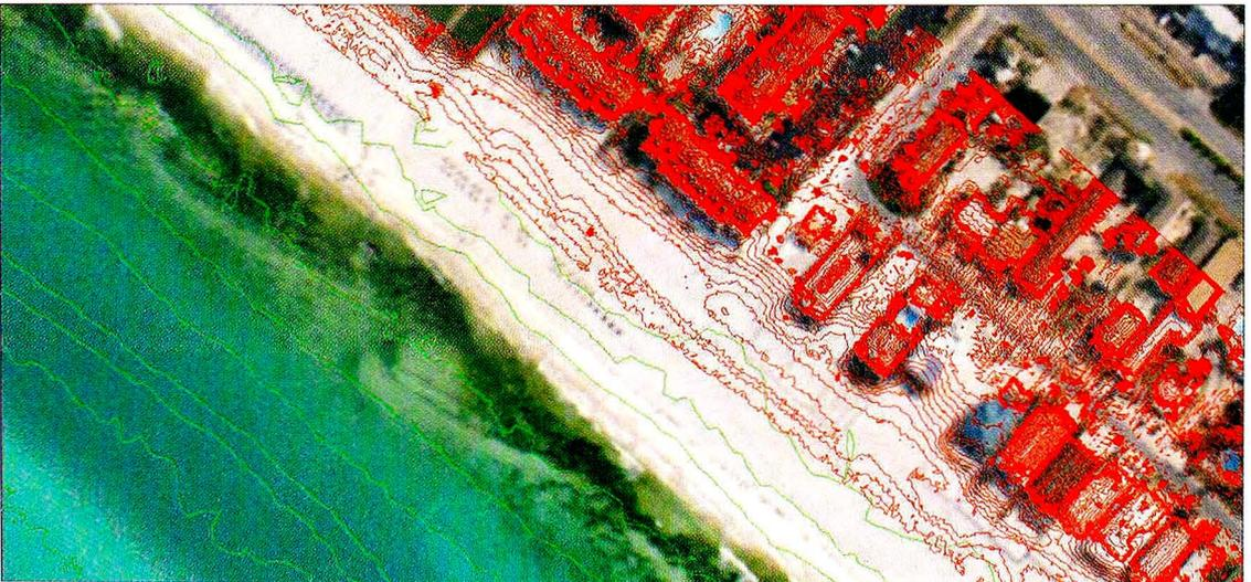
Figure 1b: Fusion of hydrographic and topographic lidar data with imagery: elevation contours
