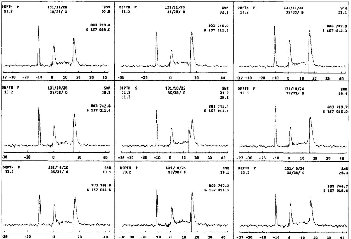
Figure 8: Display of Raw Laser Waveforms on LADS Mk II Ground System. 3x3 metre laser spot spacing. 2 metre cube target visible on central sounding (11.3 metres)
