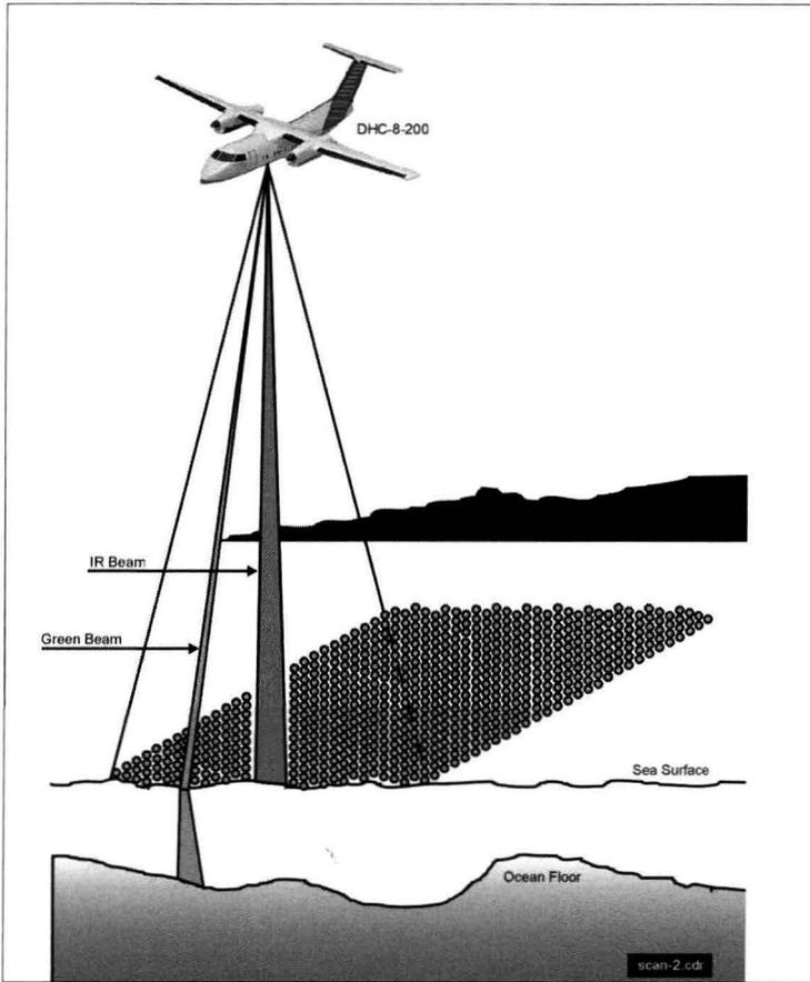
Figure 1: The laser scan
