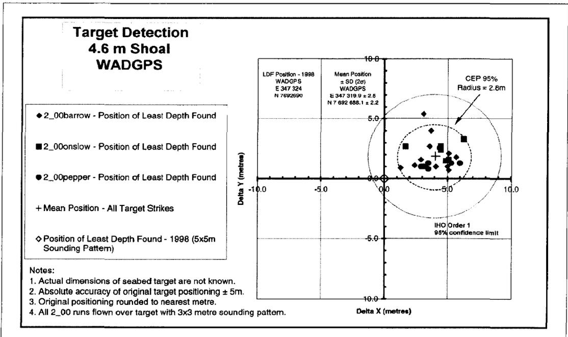
Figure 6: Detection of a well defined shoal in the survey area
