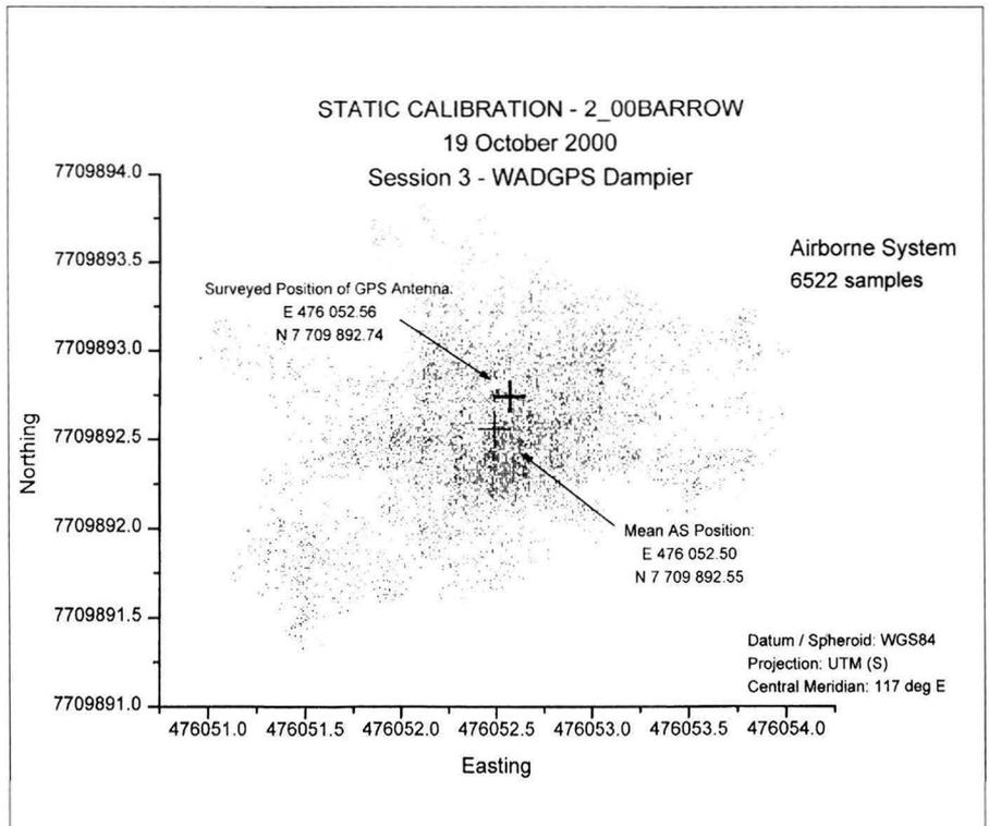
Figure 5: Scatter plot of WADGPS (Dampier)
