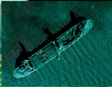
8125 multibeam data of shipwreck in the Persian Gulf, depth: 50 m
