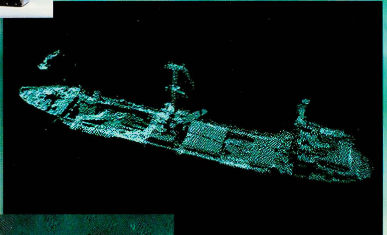
8125 multibeam data of shipwreck in the Persian Gulf, depth: 50 m
