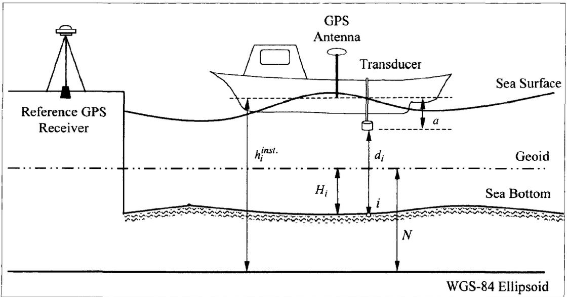
**Figure 1:** The Schematic Depiction of the Tiding the Depth to the Vertical Datum without Employing a Tide Gauge
