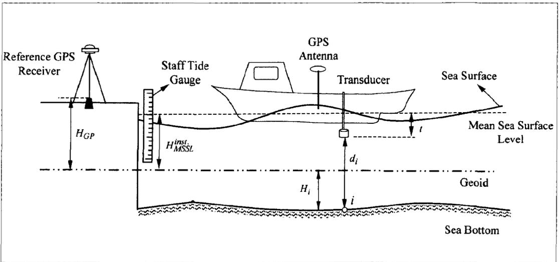
Figure 5: The Schematic Depiction of the Tiding the Depth to the Vertical Datum with Employing a Tide Gauge
