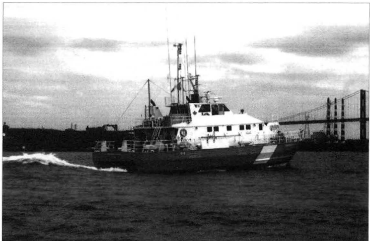
Figure 2: CCGS CREED with MVP100 on STERN
