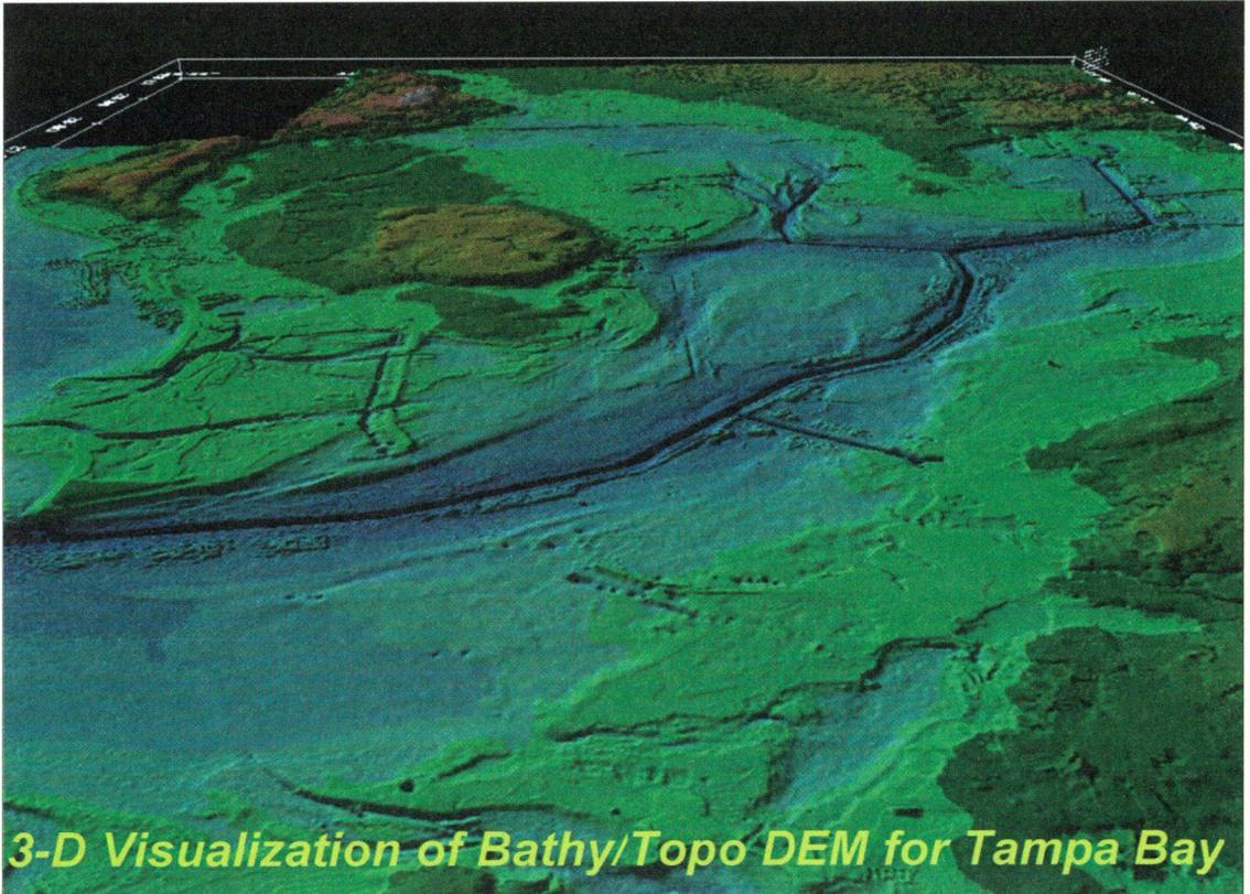
Figure 3: A 3-dimensional visualisation of the Digital Elevation Model (DEM) for Tampa Bay produced from the blending of bathymetrical and topographic data that were first transformed to a common datum using NOS' Vdatum
