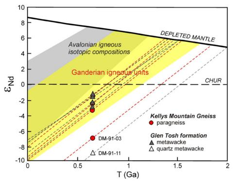
Figure 6. Plot of  $\varepsilon_{Nd}$  against time, with  $\varepsilon_{Nd}$  values calculated at 650 Ma (Table 4). The dashed lines are  $\varepsilon_{Nd}$  evolution lines, grey for metawacke samples and red for paragneiss samples. Grey shaded area indicates isotopic evolution of Neoproterozoic igneous samples from Avalonia (estimated from Murphy 2002) and overlapping yellow shaded area encloses the field for Neoproterozoic igneous samples in Ganderia estimated from Samson *et al.* (2000).
