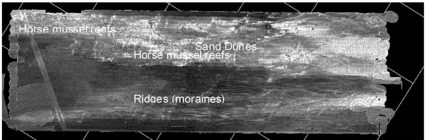
**Fig. 2.** Backscatter map of seabed reflectivity from the same region as in Figure 1. Areas of dark tone are gravel and areas of light tone represent sand. A 5.0 km grid is presented for scale. In this region of the Bay of Fundy, sand tends to dominate the northern part where the mussel reefs occur. Individual reefs are not clearly defined at this scale but show as dark-toned linear features (see Figure 6).
