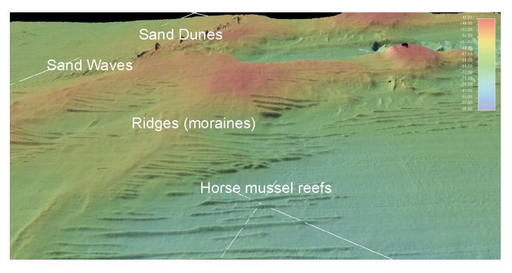
**Fig. 4.** A shaded-relief 3D image from the central area of Fig. 5, generated from multibeam bathymetric data of part of the upper Bay of Fundy centered near 45° 01'N, 65° 33'W. Depth is coded from 45 to 90 metres as shown on the attached colour bar. A 2.5 km grid has been overlain on the image for scale. Note that all of the mussel reefs in this region lie on the eastern side (right) of slight till ridges.
