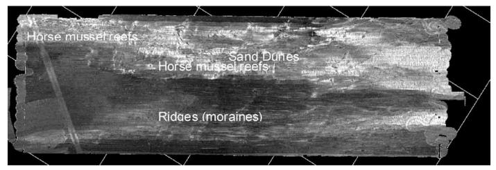
Fig. 2. Backscatter map of seabed reflectivity from the same region as in Figure 1. Areas of dark tone are gravel and areas of light tone represent sand. A 5.0 km grid is presented for scale. In this region of the Bay of Fundy, sand tends to dominate the northern part where the mussel reefs occur. Individual reefs are not clearly defined at this scale but show as dark-toned linear features (see Figure 6).
