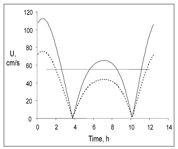
**Fig. 7.** The solid line predicts depth-averaged tidal flow in cm.s<sup>-1</sup> for one location (MG 97-20) at 44° 56.6200'N, 65° 33.7622'W in the upper Bay of Fundy, from Greenberg *et al* (2005). The dashed line predicts velocity at 6 cm above the sediment-water interface by equation below. The horizontal line suggests the limiting flow for horse mussels at 55 cm s<sup>-1</sup>.
